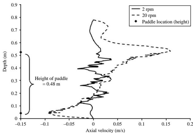
**Figure 4** | Influence of rotational speeds on the axial velocity vector profile along the depth of the flocculation tank for 2 rpm and 20 rpm.
