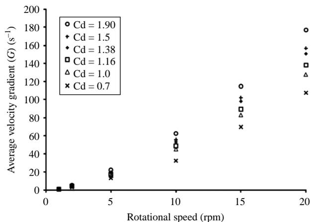
**Figure 6** | Sensitivity analysis for investigating the effect of drag coefficient values on the empirical  $G$ -value calculated.
