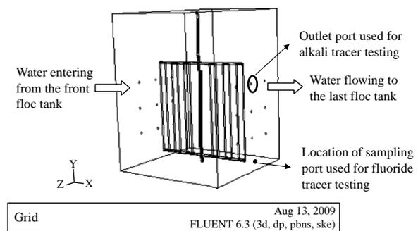
**Figure 1** | A 3D geometry showing the inlet and outlet configuration of the middle flocc tank of the three-stage paddle flocculation process of pilot-scale system at JDKWSP.
