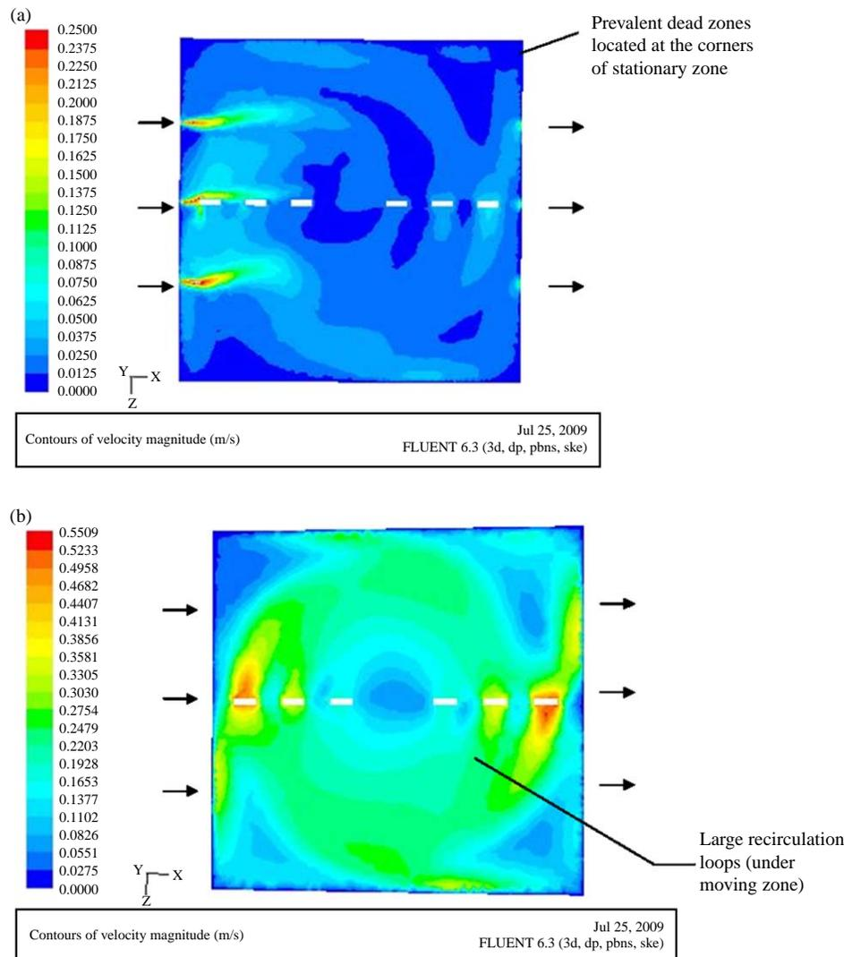
Figure 3 | Influence of rotational speeds on the contour profile of velocity magnitude along the radial plane at a mid-depth of 0.380 m of flocculation tank (a) 2 rpm (b) 20 rpm.
