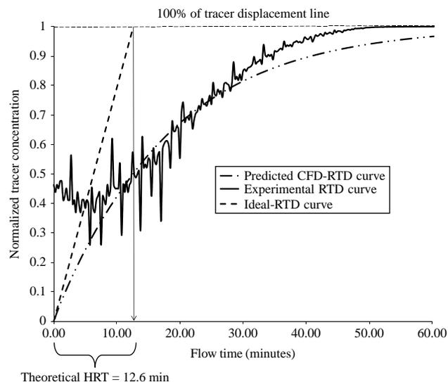
**Figure 2** | Comparison of ideal, experimental and predicted CFD-RTD curve obtained using tracer studies conducted at a rotational speed of 14.3 rpm.
