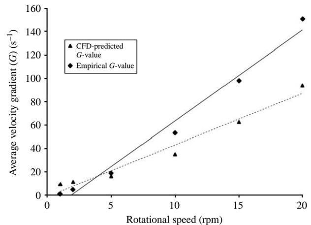
**Figure 5** | Comparison of CFD-predicted and empirical  $G$ -values for different rotational speeds for the flocculation tank.
