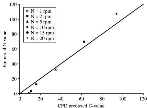
**Figure 7** | Plot of CFD-predicted and empirical  $G$ -values calculated at  $C_D = 0.7$  for different rotational speeds for the flocculation tank (line of equivalence is shown at  $45^\circ$  for reference purposes).
