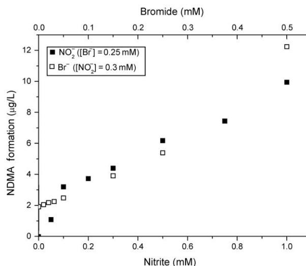
**Figure 1** | NDMA formation as a function of nitrite concentration (mM) during chlorination in the presence of 0.25 mM bromide, and as a function of bromide concentration (mM) in the presence of 0.3 mM nitrite.  $[\text{HOCl}] = [\text{DMA}] = 0.3 \text{ mM}$ ,  $\text{pH} = 7.0$ ,  $20^\circ\text{C}$ , duration of experiment 24 h.
