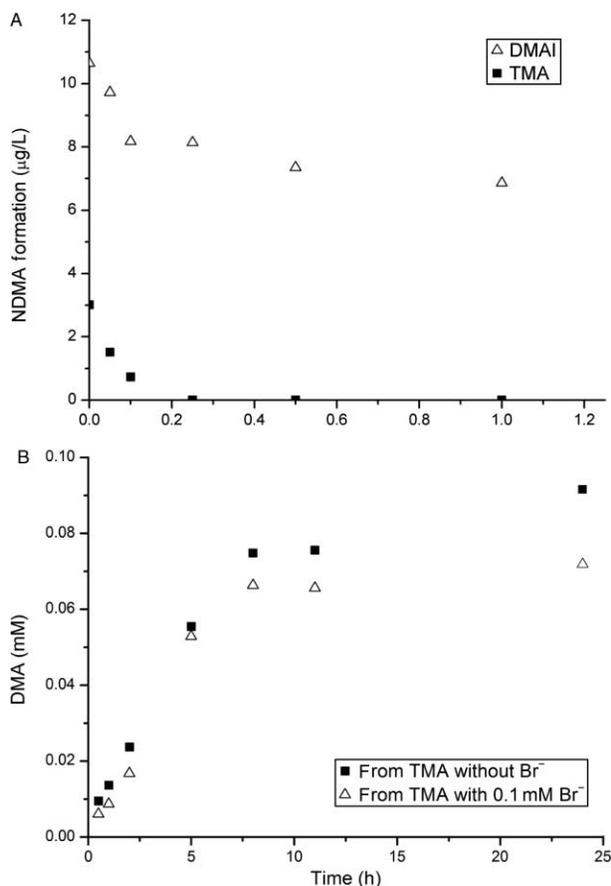
**Figure 6** | (A) NDMA formation as a function of bromide concentration during chloramination when tertiary amines were used as the organic precursors.  $[\text{NH}_2\text{Cl}] = [\text{DMAI}] = [\text{TMA}] = 0.3 \text{ mM}$ , pH = 7.0, 20°C, 24 h; (B) Formation of DMA during chloramination of TMA with and without 0.1 mM bromide.  $[\text{NH}_2\text{Cl}] = [\text{TMA}] = 0.3 \text{ mM}$ , pH = 7.0, 20°C.
