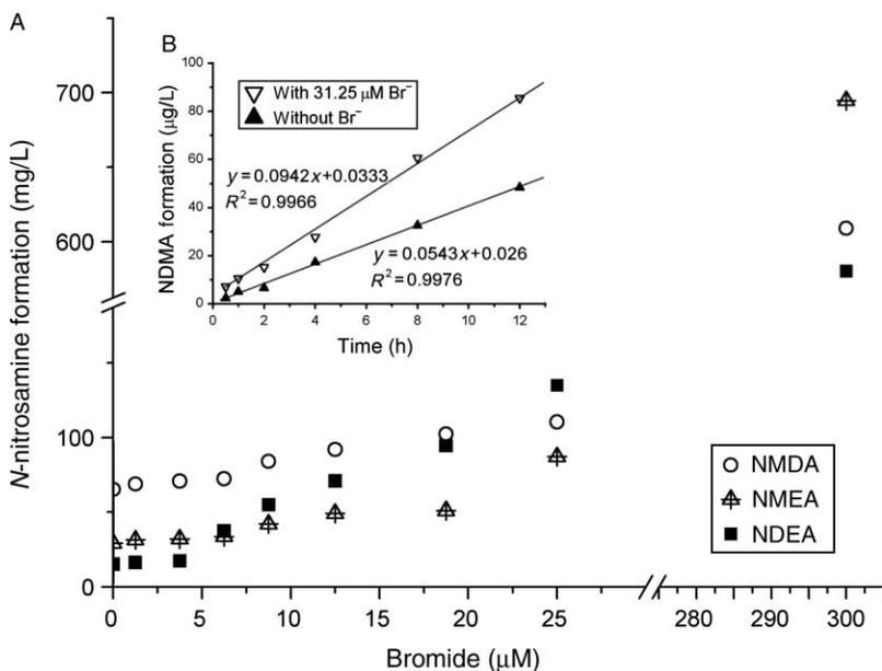
**Figure 4** | (A) Nitrosamine formation as a function of bromide concentration during chloramination.  $[\text{NH}_2\text{Cl}] = [\text{DMA}] = [\text{MEA}] = [\text{DEA}] = 0.3 \text{ mM}$ ,  $\text{pH} = 7.0$ ,  $25^\circ\text{C}$ ,  $24 \text{ h}$ ; (B) NDMA formation as a function of reaction time with and without  $31.25 \mu\text{M Br}^-$ ,  $\text{pH} = 7.0$ ,  $25^\circ\text{C}$ ,  $[\text{DMA}] = 0.3 \text{ mM}$ ,  $[\text{NH}_2\text{Cl}] = 1 \text{ mM}$ .
