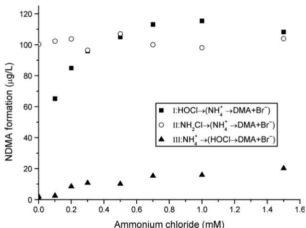
**Figure 3** | NDMA formation as a function of  $\text{NH}_4^+$  concentration during chlorination with  $31.25 \mu\text{M}$  bromide.  $[\text{HOCl}] = [\text{DMA}] = 0.3 \text{ mM}$ ,  $\text{pH} = 7.0$ ,  $25^\circ\text{C}$ ,  $36 \text{ h}$ .
