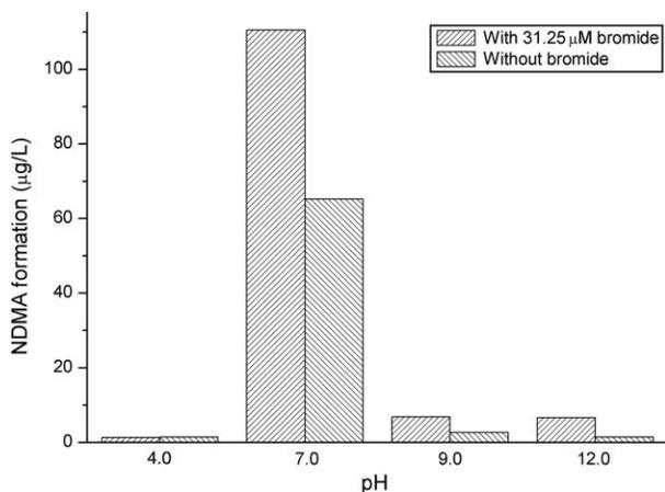
**Figure 5** | NDMA formation as a function of pH value during chloramination with and without 31.25  $\mu\text{M}$  bromide.  $[\text{NH}_2\text{Cl}] = [\text{DMA}] = 0.3 \text{ mM}$ , pH = 7.0, 20°C, 24 h.
