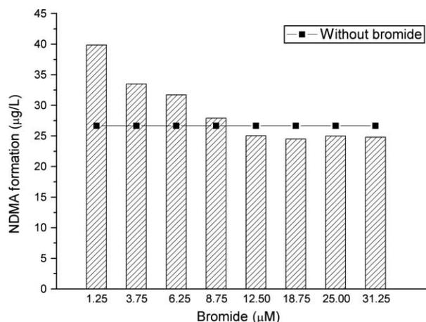
**Figure 2** | NDMA formation as a function of bromide concentration during chlorination. [HOCl] = [DMA] = 0.3 mM, pH = 7.0, 25°C, 36 h.
