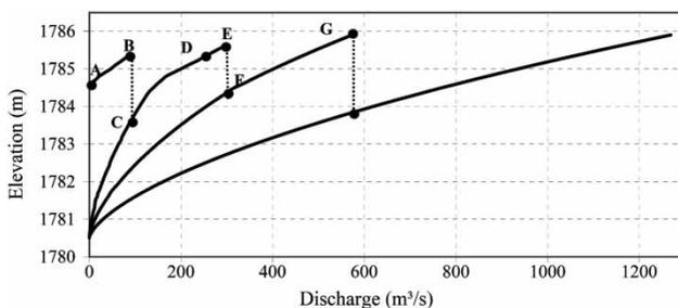
Figure 3 | Elevation–discharge curve.
