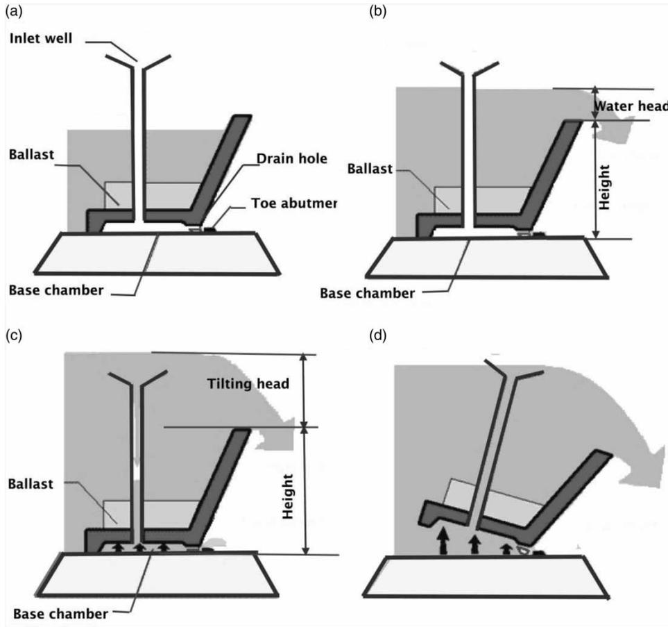
**Figure 2** | Fusegate's cross-sections through a fusegate: (a) the water level is increasing, (b) fusegate acts as an ungated spillway, (c) the water head reaches to the predetermined elevation (design tipping head), and (d) the fusegate tips (Adapted from Hydroplus site [www.hydroplus.com](http://www.hydroplus.com)).
