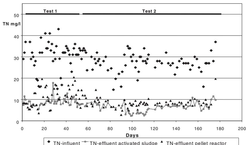
**Figure 2** Total nitrogen (TN) concentration for the classical activated sludge versus the pellet reactor during the trials. The local TN-consent is 10 mg/l (yearly average)
