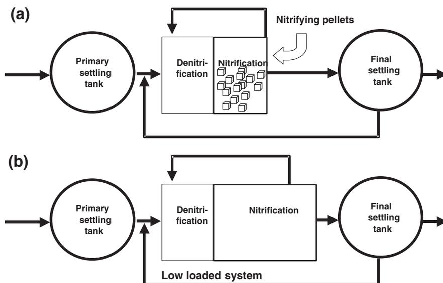
**Figure 1** Schematic representation of nutrient removing installations: (a) a high loaded entrapped nitrifier pellet reactor, versus (b) a classical low loaded activated sludge process
