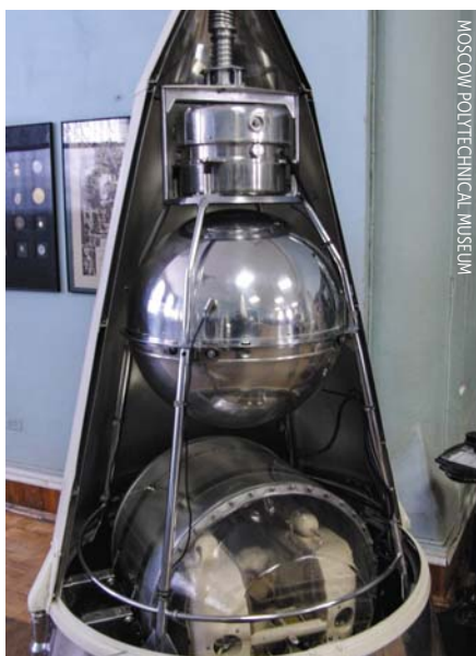
FIGURE 1. SPUTNIK 2 WAS A 4-METER-TALL, CONE-SHAPED CAPSULE designed to remain attached to the rocket that launched it into orbit on 3 November 1957. It held radio transmitters, a telemetry system, a Geiger counter, and a temperature-control system for the cabin, which carried the dog Laika. The model shown here is now at the Polytechnical Museum in Moscow.
