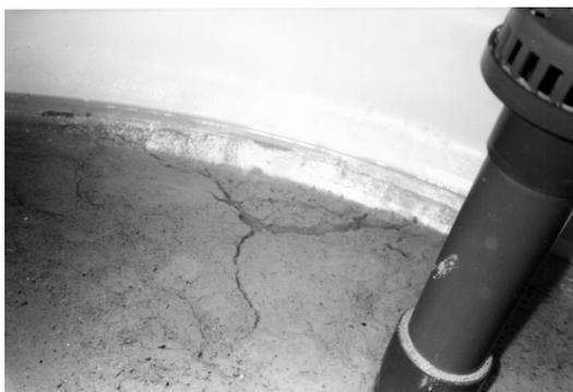
**Figure 3** The surface of the sand filter showing major fissuring
