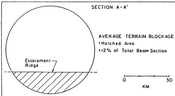
Fig. 5. The Beam Blockage.
