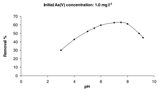
Figure 5 | Effect of pH on As (V) removal.
