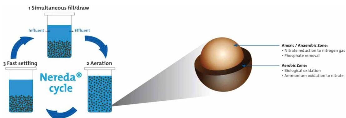
**Figure 1** | Schematic view of the Nereda® cycle.
