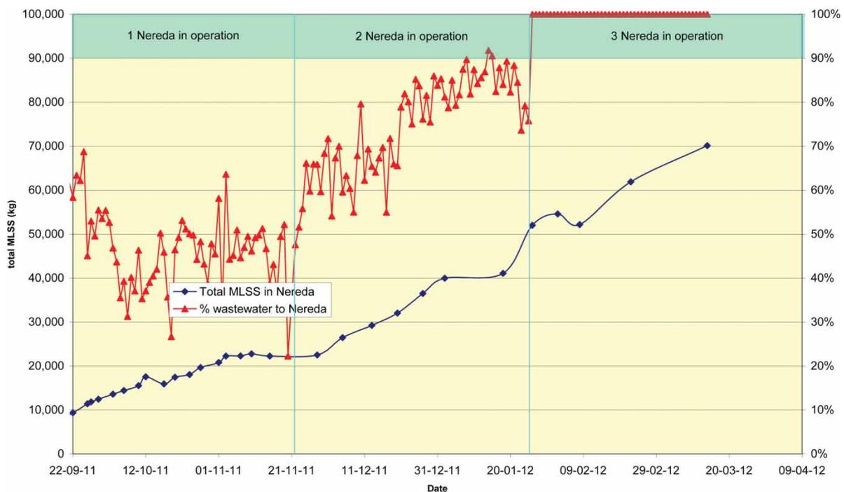
**Figure 7** | Start-up of Nereda<sup>®</sup> STP Epe.
