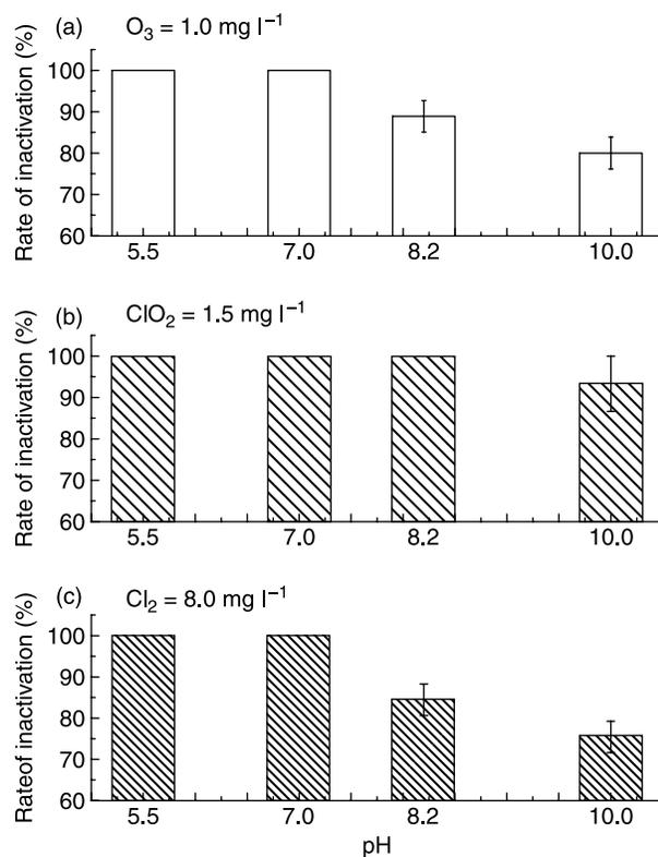
**Figure 2** | Effect of pH on inactivation of *Chironomus kiiensis* larvae with different oxidants at 25°C after reaction for 30 min.
