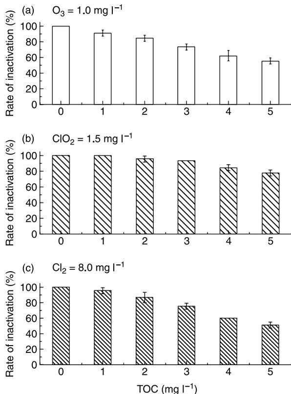
**Figure 3** | Effect of TOC on inactivation of *Chironomus kiiensis* larvae with different oxidants at 25°C and pH 7.0 after reaction for 30 min.
