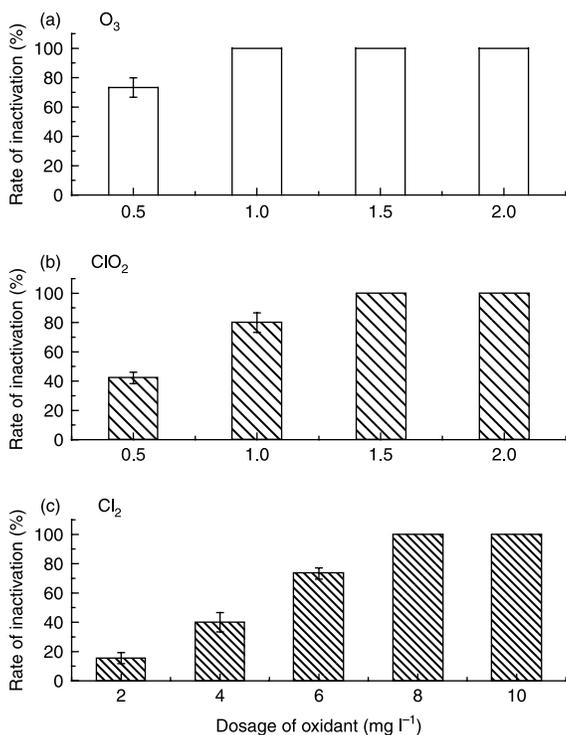
**Figure 1** | Inactivation effects of different oxidants on *Chironomus kiiensis* larvae at pH 7.0 and 25°C.
