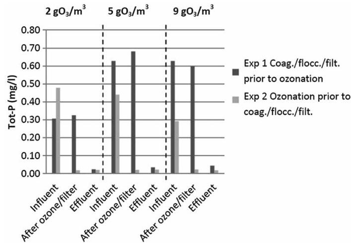
**Figure 2** | Total phosphorus (Tot-P) test results from Experiment 1 and 2; Exp. 1 Coagulation/flocculation/discfiltration prior to ozonation and Exp. 2 Ozonation prior to coagulation/flocculation/discfiltration. (mg/l).
