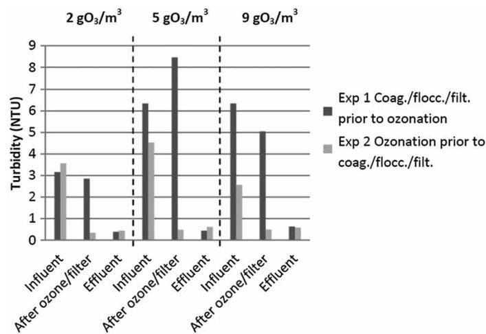
**Figure 3** | Turbidity test results from pilot experiment 1 and 2; Exp. 1 Coagulation/flocculation./discfiltration prior to ozonation and Exp. 2 Ozonation prior to coagulation/flocculation/discfiltration. (NTU).
