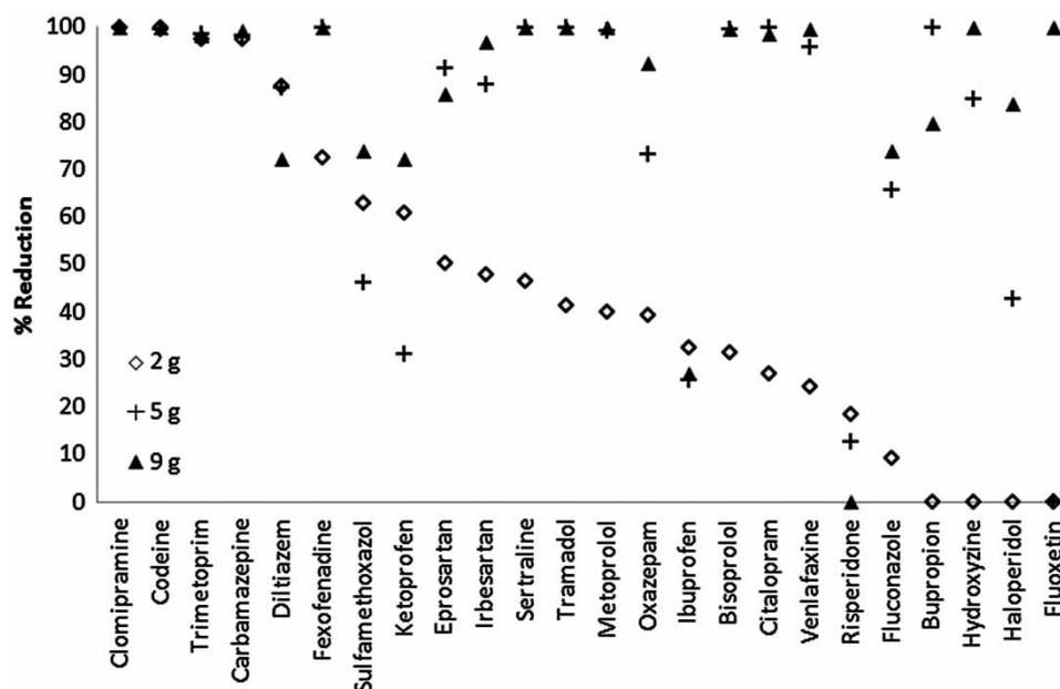
**Figure 5** | Reduction of 24 organic micro-pollutants by ozone alone for each ozone dose (2, 5 and 9 gO<sub>3</sub>/m<sup>3</sup>) in Experiment 1, ozone after discfiltration.
