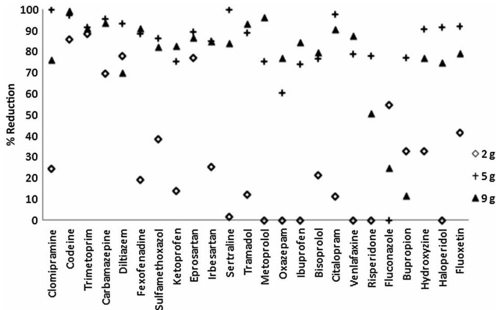
**Figure 6** | Reduction of 24 organic micro-pollutants by ozone alone for each ozone dose (2, 5 and  $9 \text{ gO}_3/\text{m}^3$ ) in Experiment 2, ozone before discfiltration.
