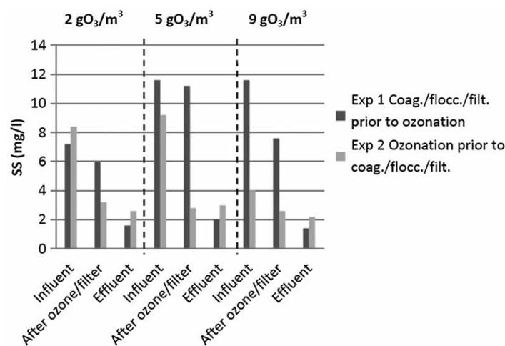
**Figure 4** | Suspended solids (SS) test results from pilot experiment 1 and 2; Exp. 1 Coagulation/flocculation/discfiltration prior to ozonation and Exp. 2 Ozonation prior to coagulation/flocculation/discfiltration. (mg/l).
