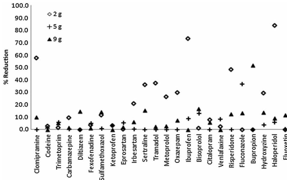
**Figure 7** | Reduction of 24 organic micro-pollutants by the coagulation/flocculation./discifiltration process for each ozone dose (2, 5 and 9 gO<sub>3</sub>/m<sup>3</sup>) in Experiment 2.
