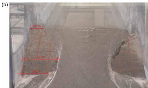
Figure 6 | Breach area (a) in Wishart (2007) model, (b) in  $t_1$  test.
