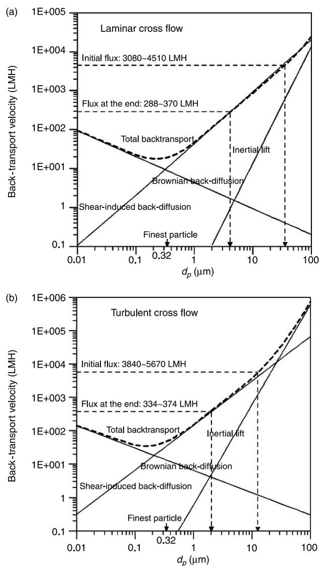
**Figure 5** | (a) The total back-transport velocity as a function of size of particulate matters deposited under laminar cross flow (the gravitational settling velocity is not depicted). (b) The total back-transport velocity as a function of size of particulate matters deposited under turbulent cross flow (the gravitational settling velocity is not depicted).
