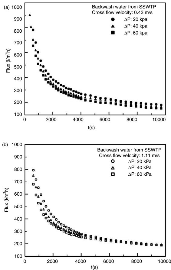
**Figure 3** | (a) The flux as affected by TMP under laminar cross flow in the case of SSWTP. (b) The flux as affected by TMP under turbulent cross flow in the case of SSWTP.
