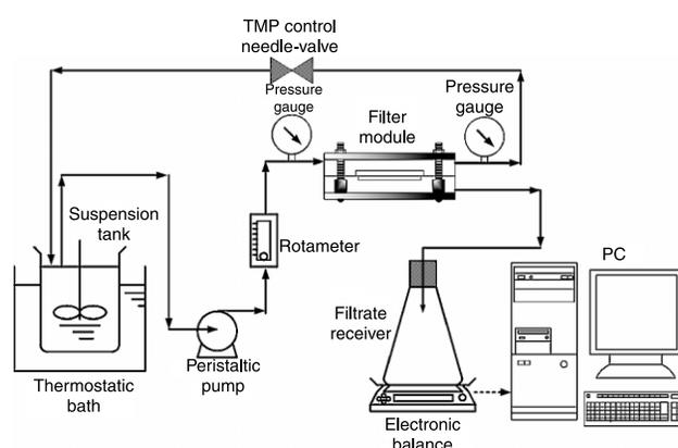
Figure 2 | Scheme of cross flow microfiltration system.
