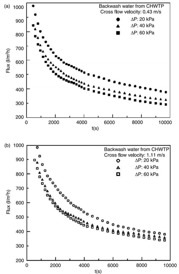
**Figure 4** | (a) The flux as affected by TMP under laminar cross flow in the case of CHWTP. (b) The flux as affected by TMP under turbulent cross flow in the case of CHWTP.
