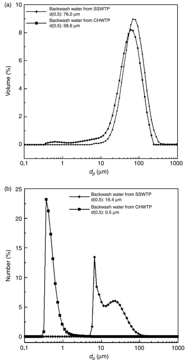
**Figure 1** | (a) Volume-based size distribution of two backwash waters. (b) Number-based size distribution of two backwash waters.
