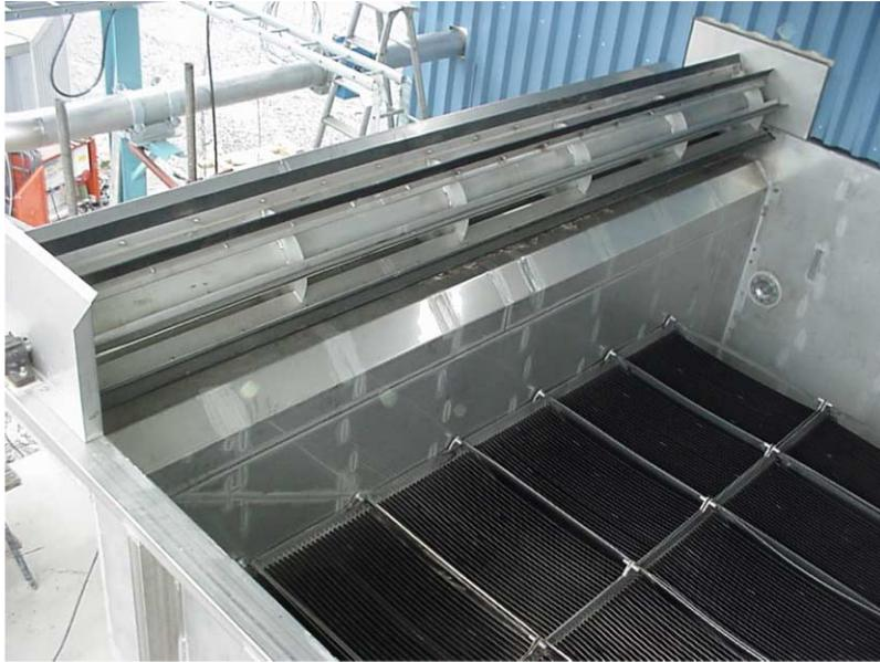
**Figure 4** | DAFRapid<sup>®</sup> unit (photo courtesy of Purac AB).
