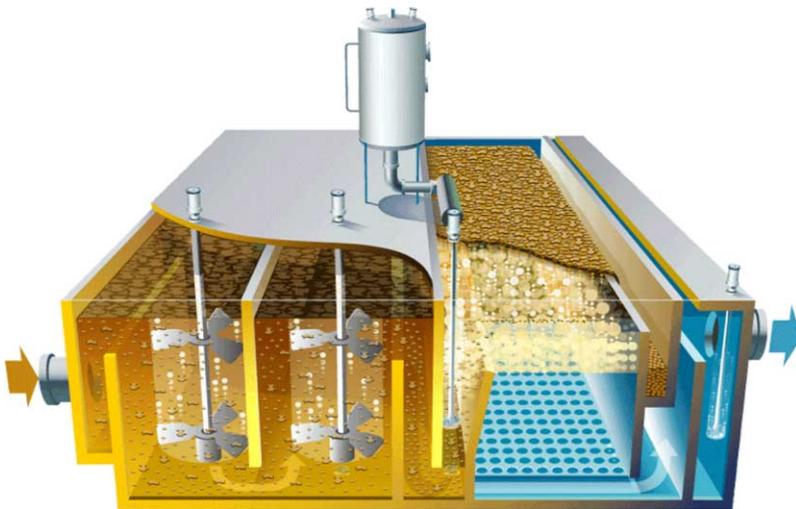
**Figure 5** | Typical AquaDAF<sup>®</sup> tank configuration (courtesy of IDI).
