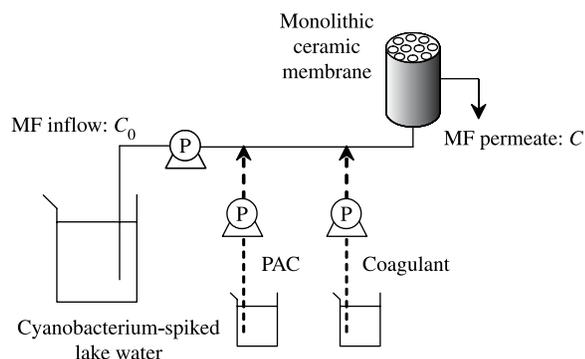
**Figure 2** | Schematic of the pilot-scale hybrid system with PAC adsorption, coagulation, and microfiltration.
