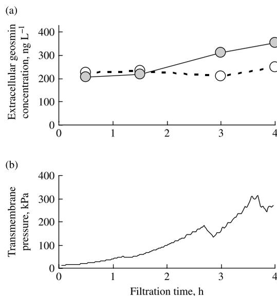
**Figure 4** | Changes in extracellular geosmin concentration in the MF inflow and in the MF permeate (a), and transmembrane pressure (b), in laboratory-scale MF experiments. White and gray circles represent the extracellular geosmin concentrations in the MF inflow and in the MF permeate, respectively.
