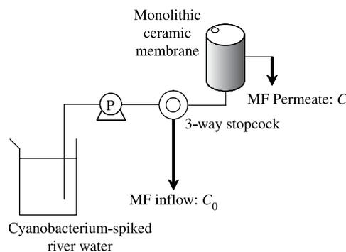
Figure 1 | Schematic of the laboratory-scale MF experiment.
