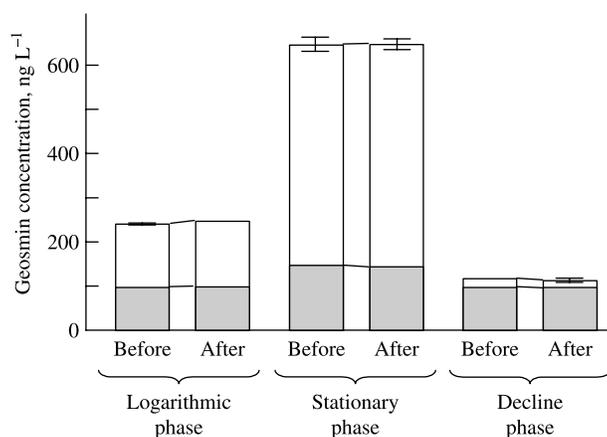
**Figure 3** | Changes in geosmin concentration before and after pressurization (400 kPa, 4 h). White and gray columns represent intra- and extracellular geosmin concentrations, respectively. Error bars represent standard deviation ( $n = 3$ ).
