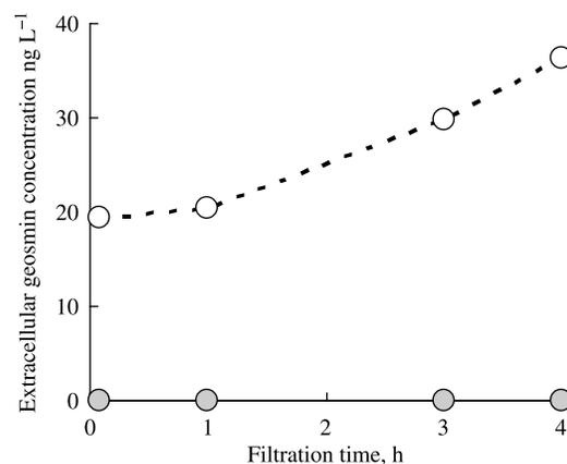
**Figure 5** | Change in extracellular geosmin concentration in pilot plant experiments with a hybrid system that used PAC adsorption, coagulation, and microfiltration. White and gray circles represent N-PAC and S-PAC addition, respectively.
