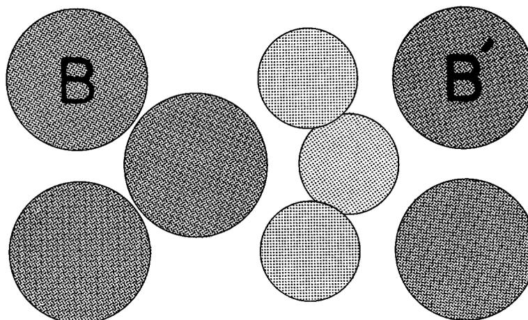
TEXT-FIG. 3. Appearance of plane through center ( $B - B'$ ) of a 200 Å thick section. The circles correspond directly to the areas of the particles in this plane. The variation in tone corresponds approximately to the variation in volume of the whole section of each particle.
