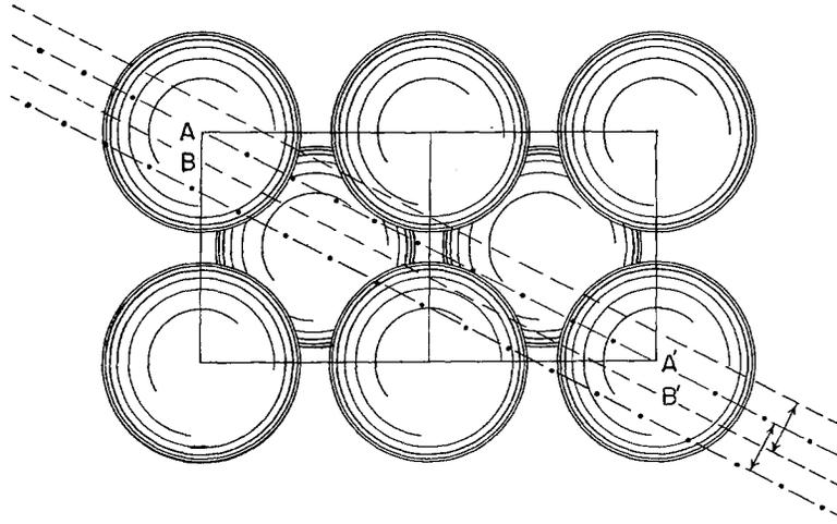
TEXT-FIG. 1. Cubic body-centered structure projected on the  $c$  plane showing the traces of two sections both parallel to the  $(120)$  plane. The width of the section corresponds to a 200 A thickness for a particle of 650 A diameter.
