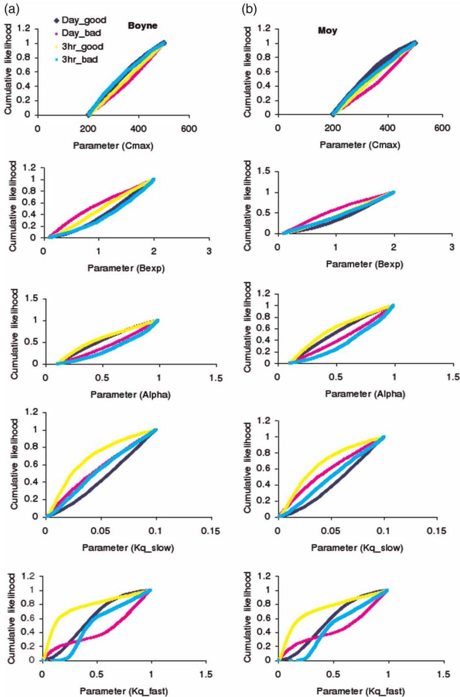
**Figure 2** | Regional sensitivity analysis plots showing the sensitivity of the parameters of the HYMOD model and its sensitivity to modelling time step for (a) Boyne river catchment and (b) Moy river catchment.
