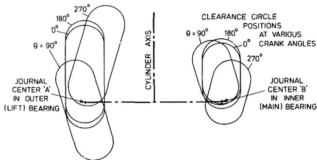
Fig. D5 Clearance space displacement for GMT 1060 engine
