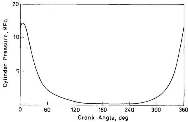
Fig. C2: Typical cylinder pressure:  $p_{GAGE}$  versus  $\theta$  (Numerical example)
