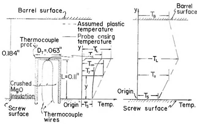
**Fig. 5** Quantities and distributions involved in the determination of average plastic temperatures
