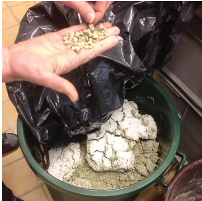
A FINNISH SCIENTIST HOLDS absorbent clay that the waste-management company Posiva Oy is considering using to backfill the tunnels before its Olkiluoto repository site is sealed and abandoned around 2120. A similar clay that also absorbs groundwater and swells will be used to snugly encase fuel-rod-containing canisters in their tombs deep underground.
