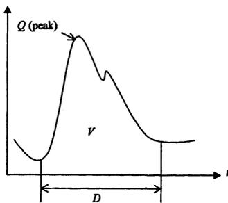
Fig. 1. Characteristic values of a flood event.
