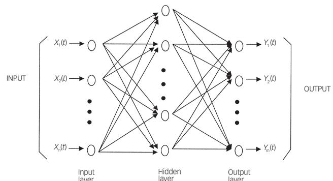
**Figure 1** | Structure of an artificial neural network.
