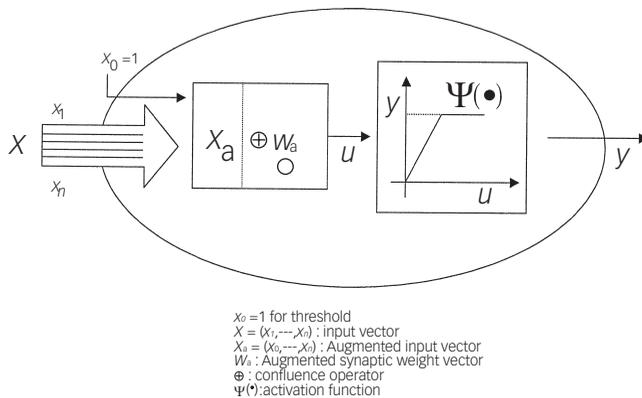
**Figure 2** | Structure of an artificial neuron.
