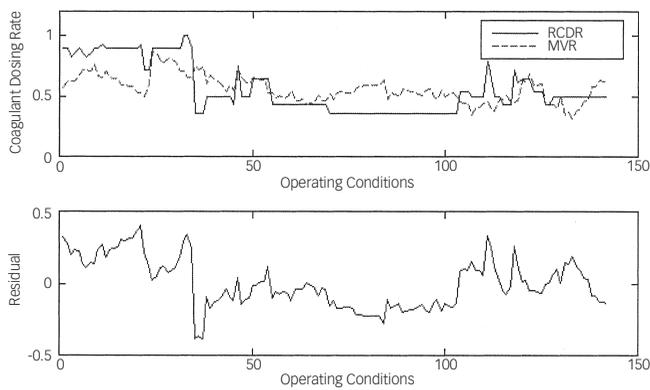
**Figure 5** | Comparison of predicted (MR) and real injection rate (RCDR) (top) and the residual (bottom) of multi-variable regression for data used in regression.
