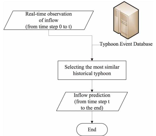
Figure 4 | The flowchart of real-time inflow forecasting.
