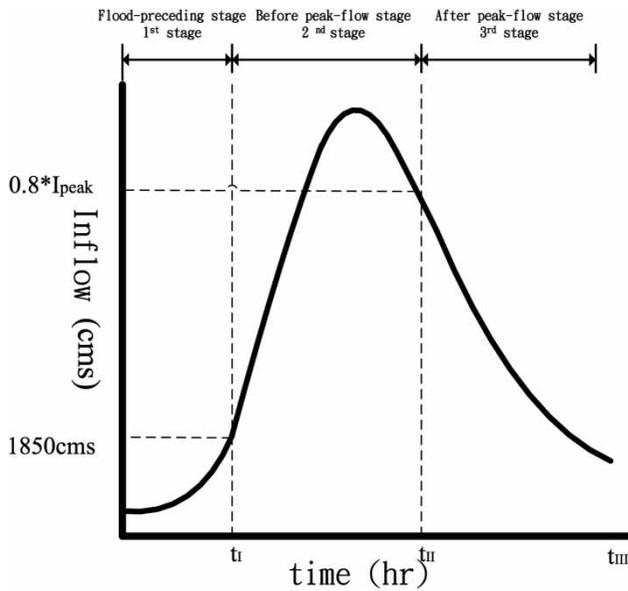
Figure 3 | The schematic of flooding operation rules.
