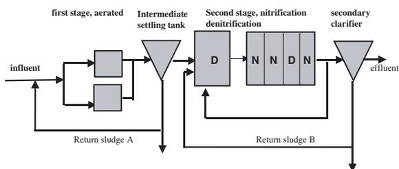
**Figure 1** Flow sheet of WWTP Cologne – Langel
