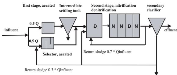
**Figure 2** Integration of the aerobic selector
