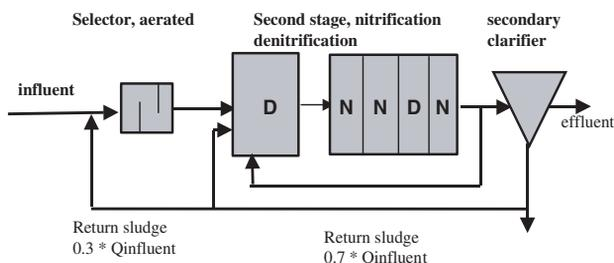
**Figure 3** Aerobic selector receiving complete waste water influent (pilot plant)
