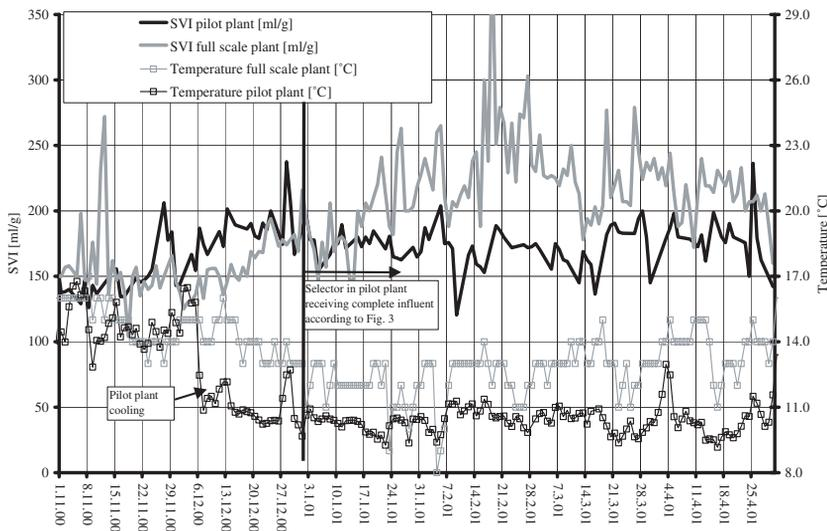
**Figure 4** SVI in full scale and pilot plant
