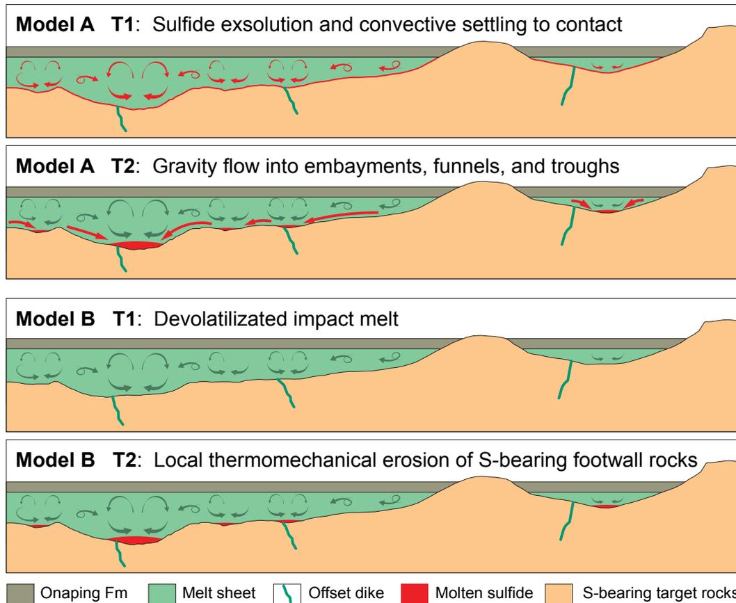
Fig. 2. Schematic representations of end-member sulfide generation and localization models. Model A: Exsolution and convective settling of molten sulfide droplets (T1) followed by gravity flow into embayments, troughs, and funnels (T2). Model B: Volatilization of most of the S from the impact melt (T1) followed by generation of sulfide xenomelts by local thermomechanical erosion (T2).
