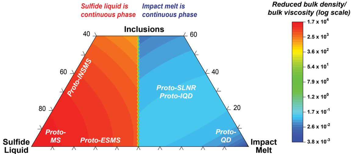
Fig. 5. Calculated reduced density/viscosity ratios of mixtures of impact melt, inclusions, and sulfide melt. Methods given in the Appendix. ESMS = emulsion semimassive sulfide, INSMS = inclusion semimassive sulfide, IQD = inclusion quartz diorite, MS = massive sulfide, QD = quartz diorite, SLNR = sublayer norite.
