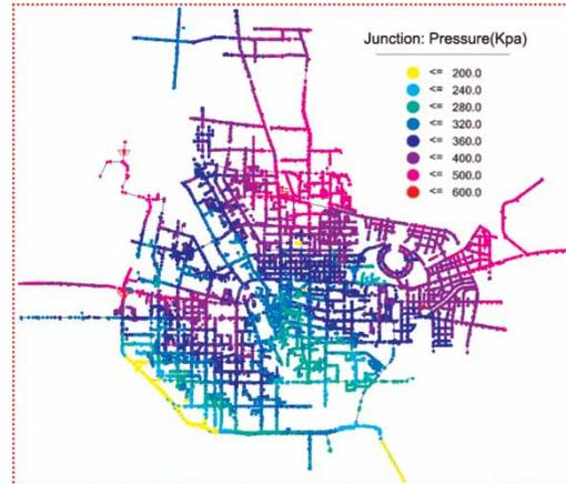
Figure 2 | Zhengzhou water distribution system pressure.
