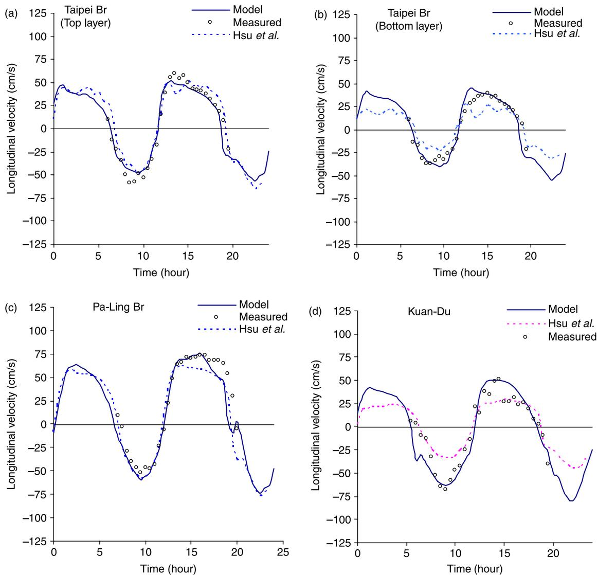
**Figure 3** | Comparison of measured and simulated longitudinal surface velocities on 24 June 1994 at (a) Taipei bridge (surface layer); (b) Taipei bridge (bottom layer); (c) Pa-Ling bridge (surface layer); and (d) Kuan-Du station (bottom layer).
