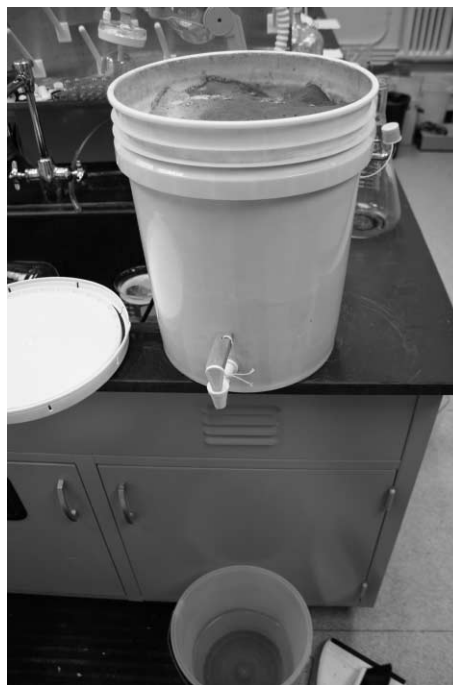
Figure 1 | Sand filter design.
