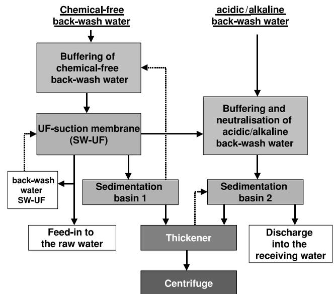
Figure 7 | Flow chart of the planned back-wash water treatment.
