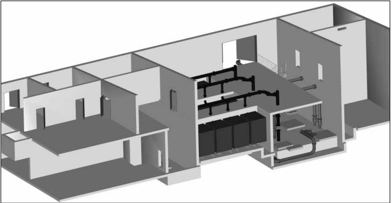
**Figure 8** | Model of the new building for the treatment of back-wash water.
