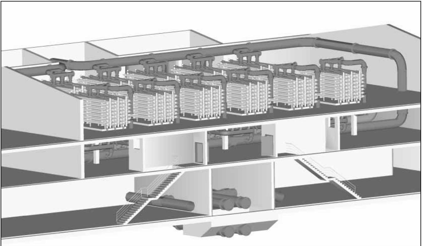
**Figure 5** | Design draft for the new part of the building of the pressure pipe versions below the new drinking water storage.
