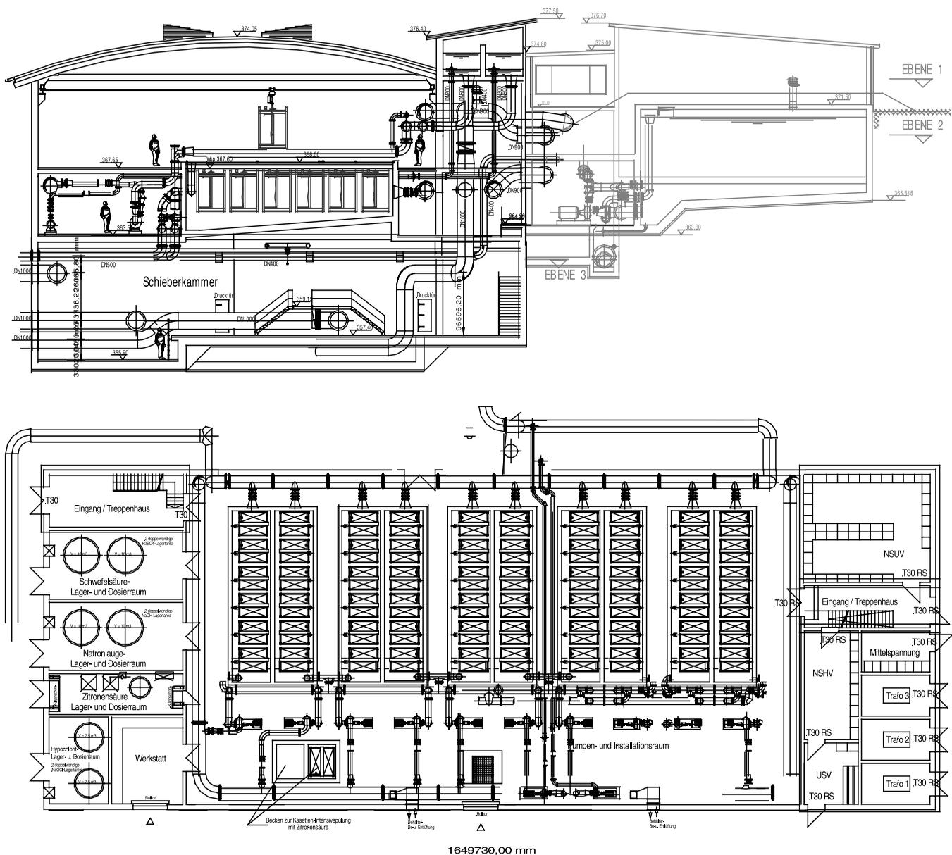
Figure 6 | Ground sketch and sectional view of the new part of the building showing the suction membrane variant above the new drinking water storage facility.
