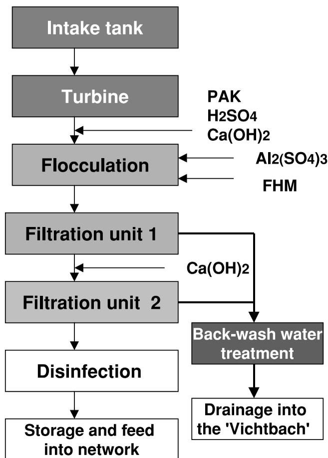
Figure 1 | Process concept of the present TWA Roetgen.
