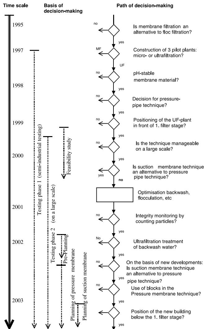
**Figure 2** | Overview of the project phases and decision-making in the planning of the extension to the TWA Roetgen (Dautzenberg *et al.* 1998, 2001; Hagemeyer *et al.* 2001; Urban & Holy 2002).
