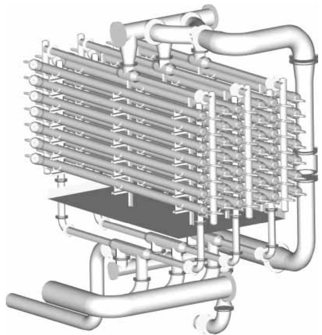
Figure 4 | Block for the pressure membrane filtration in the TWA Roetgen.
