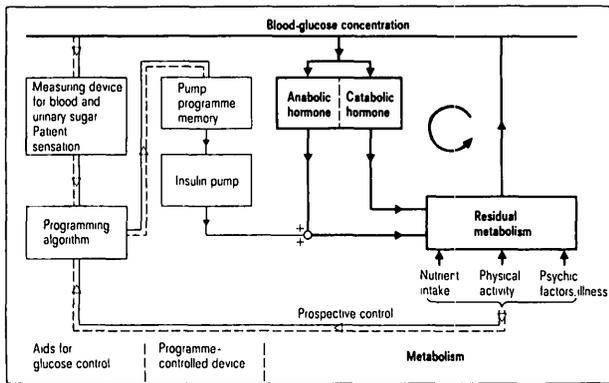
FIG. 2. Schematic diagram of the program-controlled dosing device and its linkage with the metabolic control loop.
