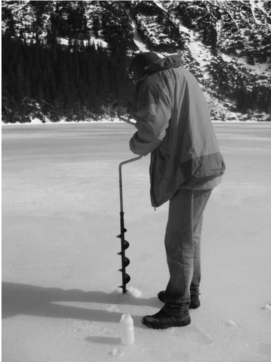
Figure 3 | Drilling before ice thickness measurements (Photo. J. Pociask-Karteczka).
