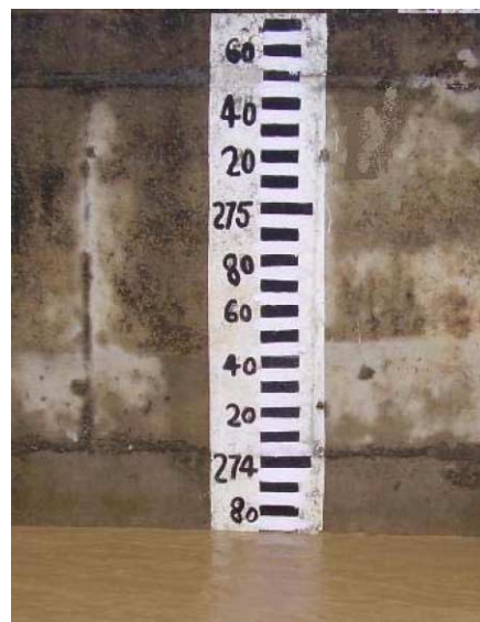
Figure 7 | Manual stage recorder at the gauging station of the Pathri Rao watershed.
