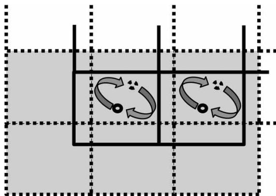
**Figure 3** | Scheme of the two-way exchange of variables between BRAMS and MGB-IPH computational cell centers. An algorithm selects the nearest computational cell centers before exchanging the coupling variables.
