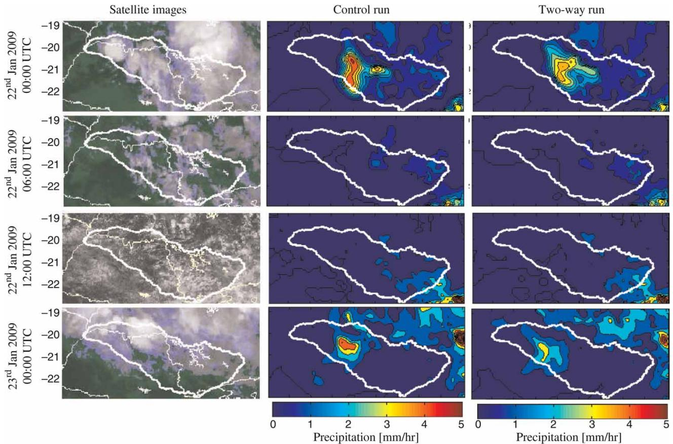
**Figure 5** | Simulated precipitation fields at 00:00, 06:00, 12:00 UTC 22 January and 00:00 UTC 23 January for the BRAMS model without any changes (control run), with the two-way coupling (two-way run), and with the water vapor observations from GOES-10. The marked line indicates the Rio Grande basin (see online version for colours: <http://www.iwaponline.com/nh/toc.htm>).
