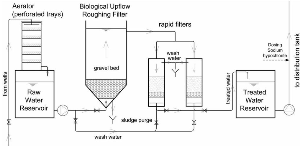
Figure 6 | Scheme of biological upgraded water treatment plant for Fe and Mn removal.
