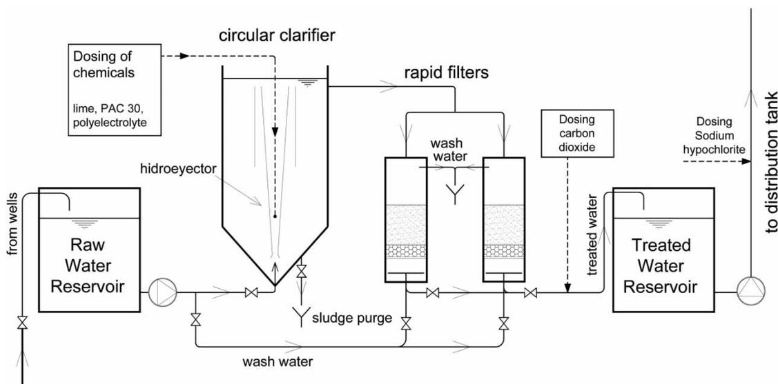
Figure 1 | Scheme of the treatment plant with physicochemical removal of Fe and Mn.
