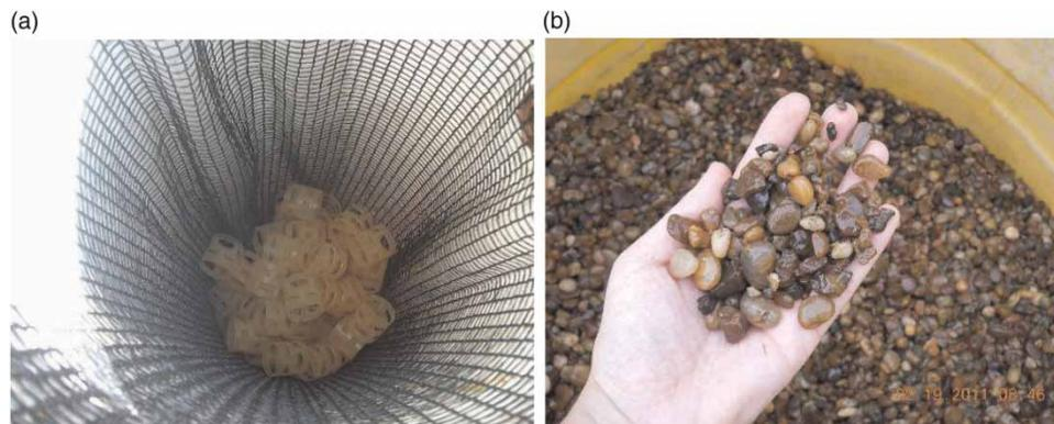
**Figure 3** | (a) Plastic rings used in the pilot tests. (b) Filtering material (gravel) used in pilot roughing filter (Steps 5–7).
