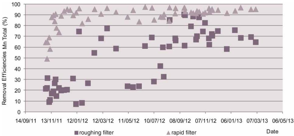
**Figure 11** | Total Mn removal efficiencies at the outlet of each stage of treatment plant.
