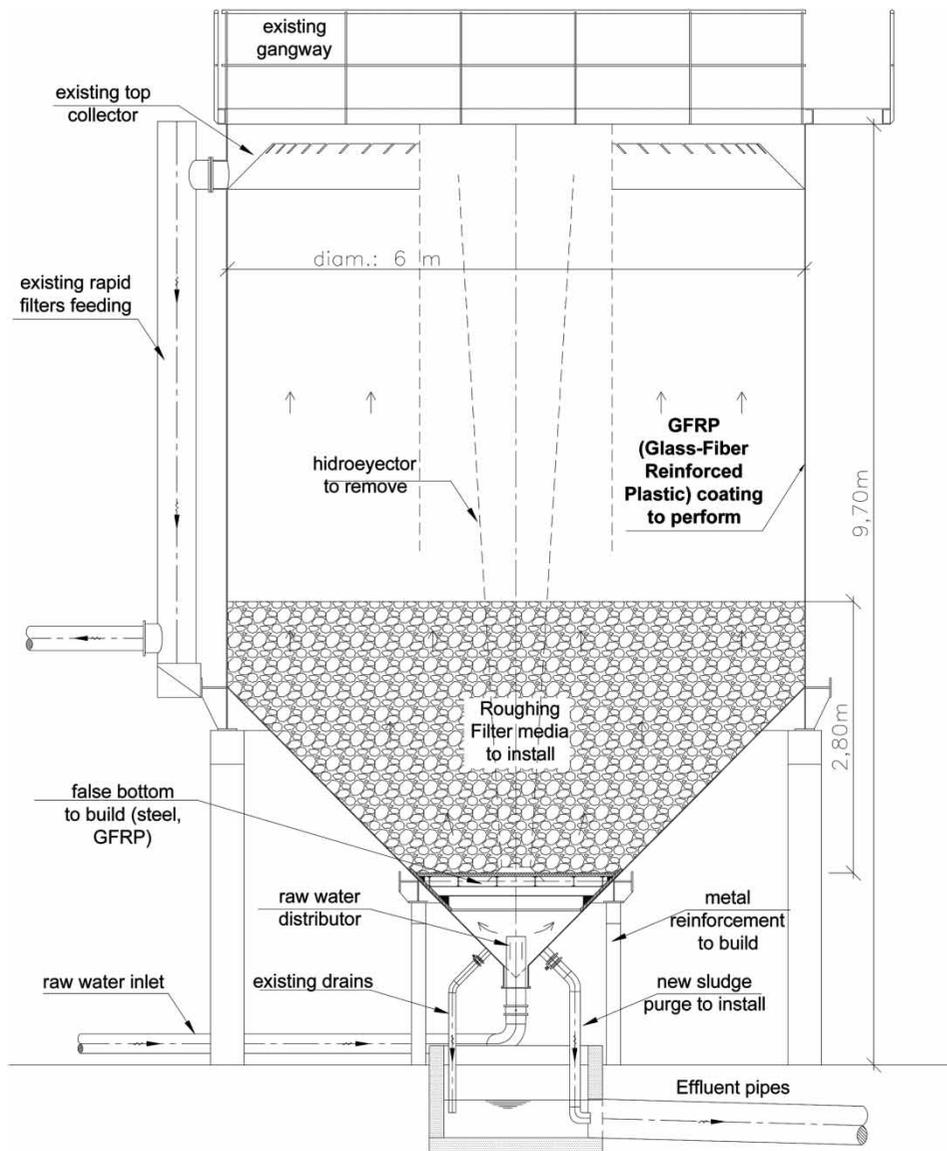
**Figure 8** | Changes made in the existing circular settler to transform it in an up-flow roughing filter.
