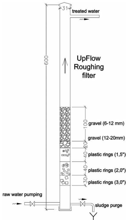
**Figure 2** | Scheme of the pilot roughing filter and the filter layers (Steps 6 and 7, see Table 1).
