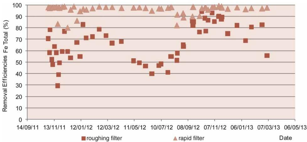
**Figure 10** | Total Fe removal efficiencies at the outlet of each stage of treatment plant.
