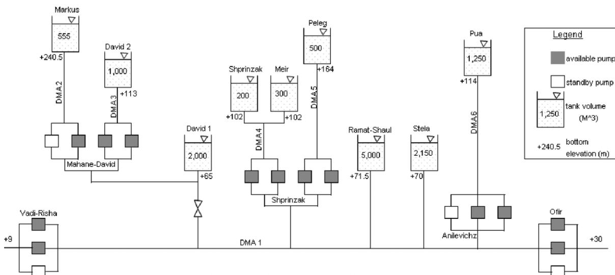
Figure 2 | Schematic representation of the Haifa-A network.
