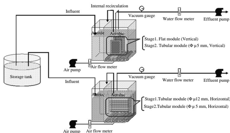
Figure 2 Schematic diagram of the experimental apparatus
