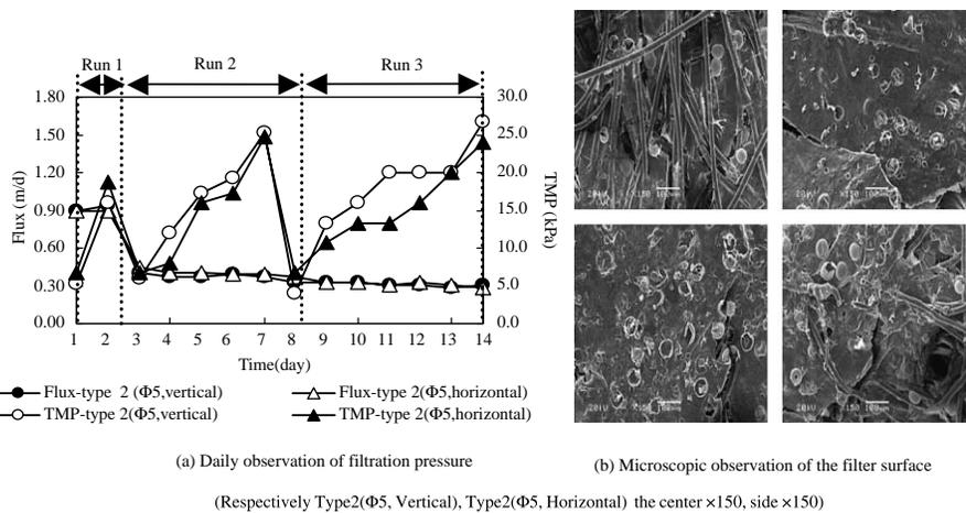
**Figure 6** Comparison of filtration pressure of the tubular filter in different installations
