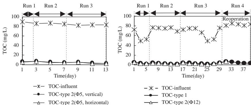
**Figure 7** Daily observation of TOC removal by the system with different types of filter module
