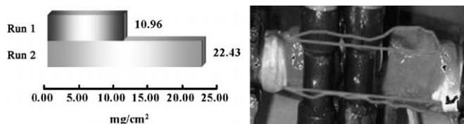
**Figure 4** Comparison of the sludge accumulated on the filter module
