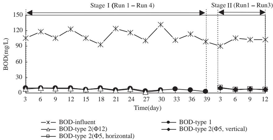
**Figure 8** Daily observation of BOD removal by the system with different types of filter module
