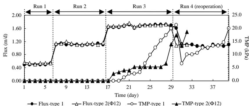
**Figure 3** Comparison of filtration pressure increase at different flux levels between the flat plate and the tubular type filter module
