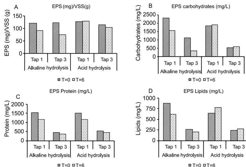
**Figure 3** Total EPS (A) and main EPS fractions identified as carbohydrates (B), proteins (C) and lipids (D) from anaerobic sludge samples at tap 1 (0.25 m) and tap 3 (1.25 m) from UASB reactor of WWTP-UFES submitted to alkaline and acid hydrolysis. n = 6; T = hours
