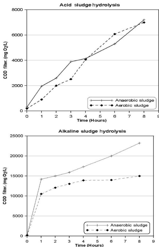
**Figure 2** Hydrolysis data from aerobic and anaerobic sludge hydrolysis with 5% TS and 20 meq/L in acid ( $H_2SO_4$ ) and alkaline (NaOH) conditions during 8 hours, expressed as COD filtered (mg O<sub>2</sub>/L)
