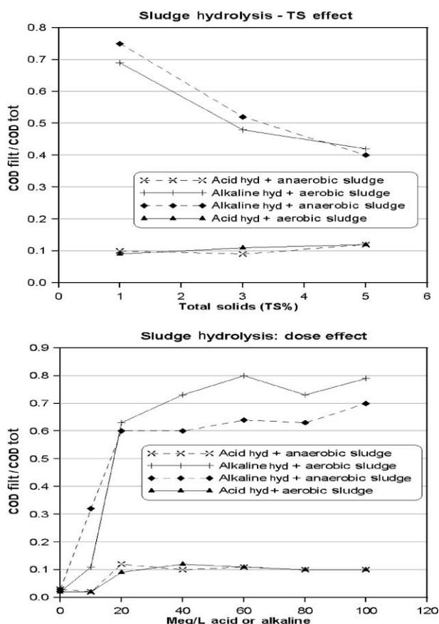
**Figure 1** Effect of sludge solubilization expressed as COD filt/COD total as a function of TS% and fixed 40 meq/L of hydrolytic agent and effect of hydrolytic agent concentration of 0–100 meq/L with fixed 1.0% TS for aerobic and anaerobic sludge after 8 hours of hydrolytic processing
