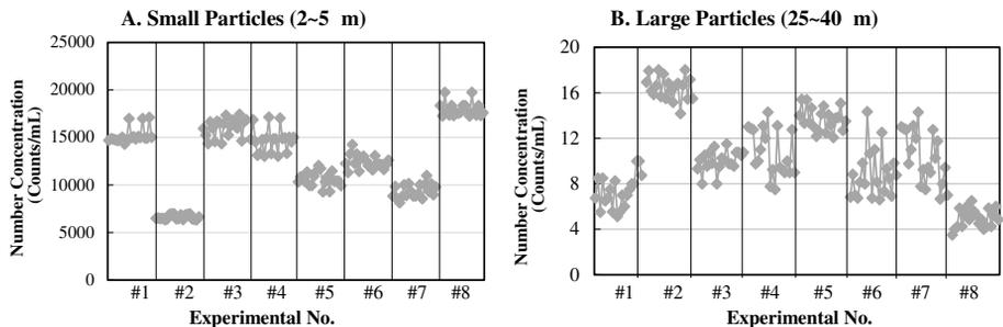
**Figure 8** Variation of number of small and large particles at each experimental condition (# represents the experiment number as shown in Table 2)
