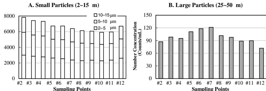
**Figure 5** Number concentration of small and large particles at distribution channel (# represents the flocculation basin as shown in Figure 4)
