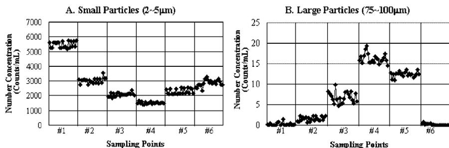
**Figure 2** Number concentration of small and large particles at each process (# represents the sampling points as shown in Figure 1)
