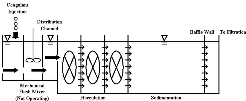
**Figure 6** Schematic diagram of Shaewoon WTP
