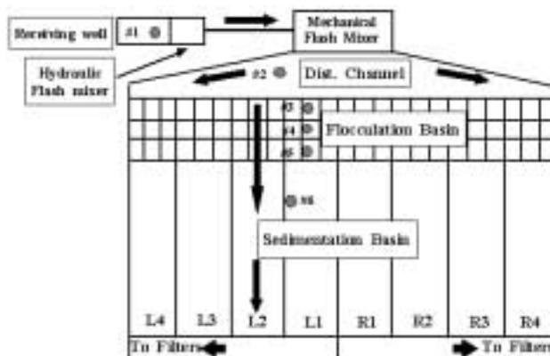
**Figure 1** Layout of Sungnam WTP (not drawn to scale)
