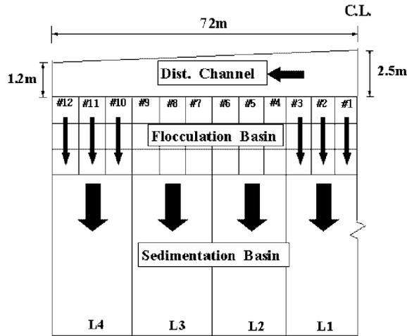
**Figure 4** Layout of distribution channel
