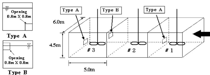
**Figure 3** Flocculation basin details of Sungnam WTP
