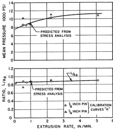
FIG. 8 MEASURED AND PREDICTED MEAN PRESSURE AS A FUNCTION OF EXTRUSION RATE
