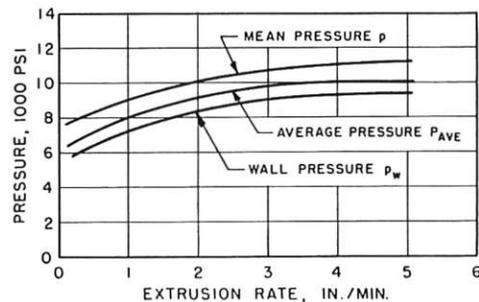
FIG. 9 COMPARISON BETWEEN MEAN PRESSURE, WALL PRESSURE, AND AVERAGE PRESSURE AS FUNCTIONS OF EXTRUSION TIME
