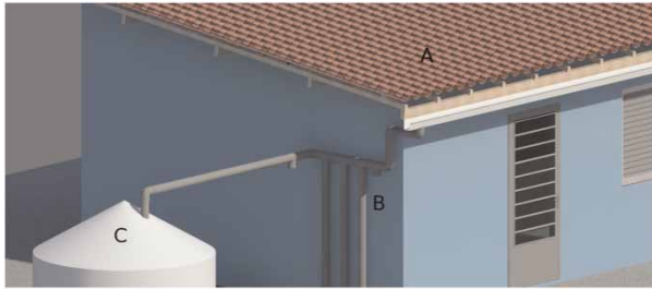
Figure 2 | Schematic illustration of the harvesting system. A: ceramic roof; B: first flush diverter; C: cistern.
