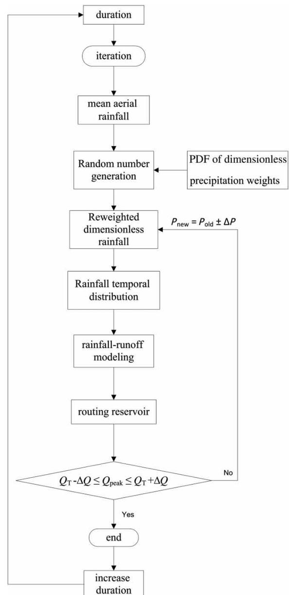
Figure 4 | Flowchart of RT extraction algorithm.
