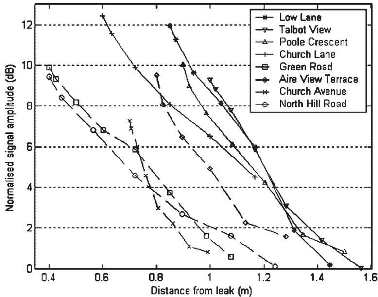
**Figure 7** | The variation in RMS signal amplitude with increasing distance from the leak; a 180 Hz high pass filter has been applied. These data are from loggers positioned parallel to and directly above the pipe. The amplitudes are given in decibels (dB). Far away from the effects of the leak the dB ratio should be zero. The greatest RMS signal amplitude is seen directly above the leak and this drops away with increasing distance from the leak.
