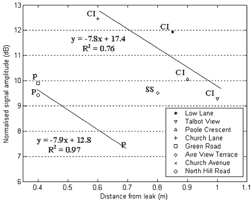
**Figure 8** | The RMS signal amplitude from the loggers positioned on the ground at a point directly above the leak position. The data from cast iron pipes (CI) and plastic pipes (P) show a decrease in amplitude with an increase in the depth of the pipe. There is only a single stainless steel pipe (SS). Trend lines for the cast iron pipes and the plastic pipes are shown with regression equations and  $R^2$  values.
