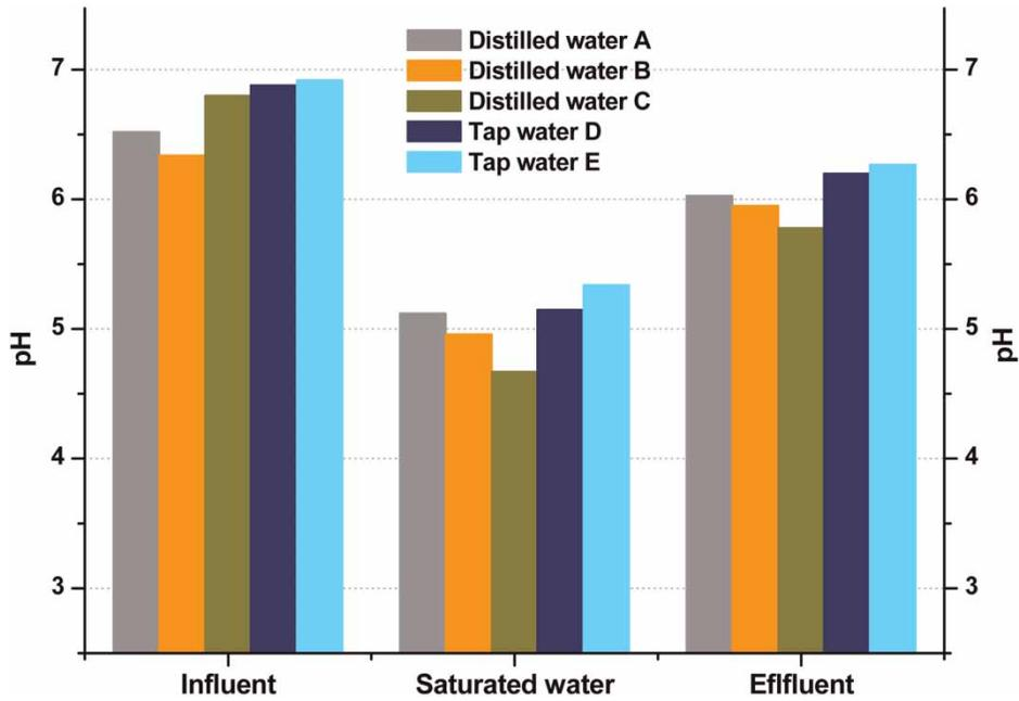
Figure 6 | Change of pH by carbon dioxide bubbles of saturated water in flotation column. (Operation condition: recycle ratio 10% (V/V),  $P_s$  151.99 kPa.)
