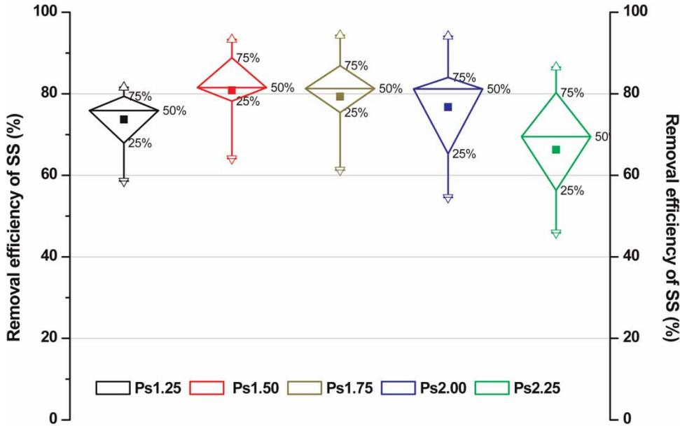
Figure 9 | Removal efficiency of SS depending on saturator pressure. (Operation condition: influent SS 84.2 mg/L, recycle ratio 10%.)
