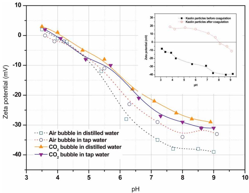
Figure 7 | Zeta potential for before and after coagulation in terms of pH.
