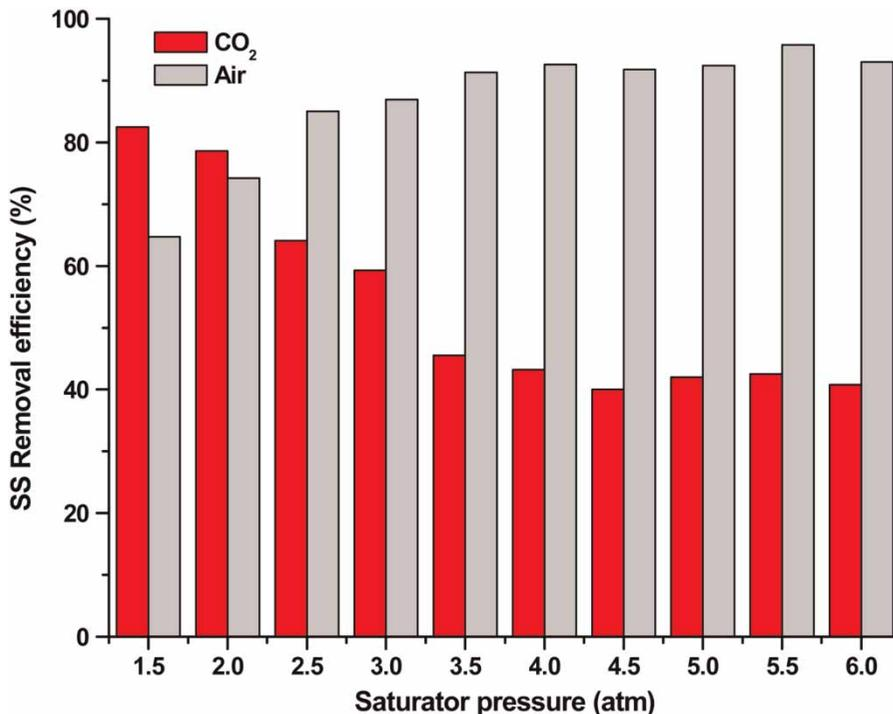
Figure 2 | Comparison of SS removal efficiency between CO<sub>2</sub> bubbles and air bubbles.
