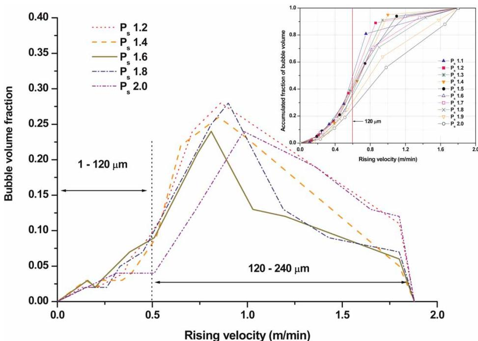
**Figure 8** | Variation of bubble volume fraction depending on saturator pressure.
