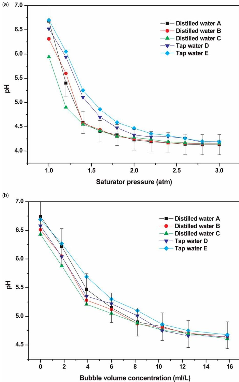
Figure 5 | Change of pH by carbon dioxide bubbles in saturation tank. (a) Saturator pressure (BVC 4.5 ml/L); (b) bubble volume concentration ( $P_s$  151.99 kPa).
