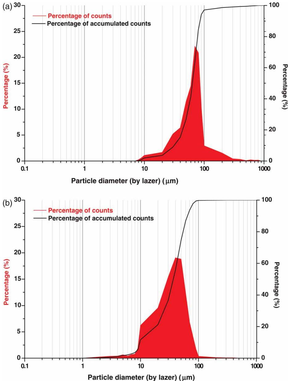
**Figure 3** | Bubble diameter distribution in flotation column. (a) CO<sub>2</sub> bubbles, (b) air bubbles.
