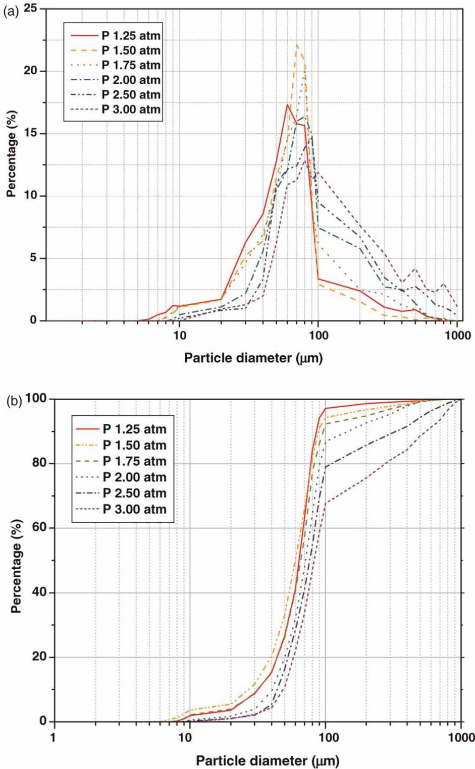
Figure 4 | CO<sub>2</sub> bubble diameter distribution in terms of saturator pressure. (a) Percentage of bubble counts; (b) accumulated percentage of bubble counts.
