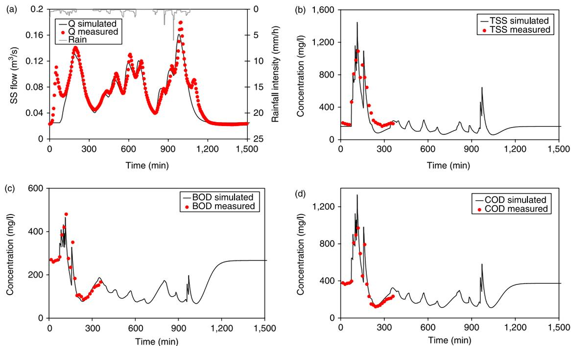
**Figure 5** | Comparison between monitored data and modelling outputs at the Montelepre SS outlet (event 5/03/2008): (a) rainfall pattern and SS outflow discharge; concentrations of TSS (b), BOD (c) and COD (d).
