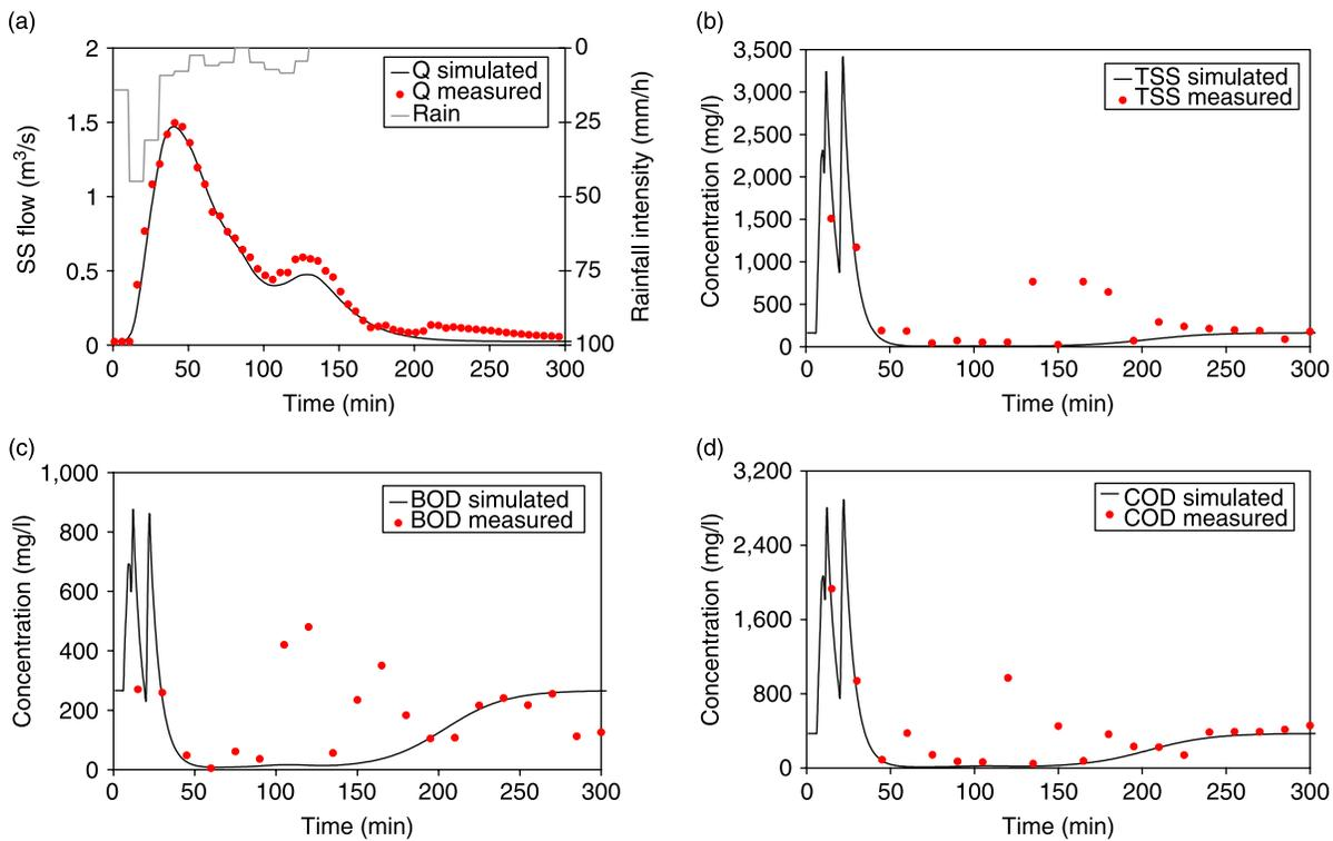
**Figure 8** | Comparison between monitored data and modelling outputs at the Giardinello SS outlet (event 27/04/2008): (a) rainfall pattern and SS outflow discharge; concentrations of TSS (b), BOD (c) and COD (d).
