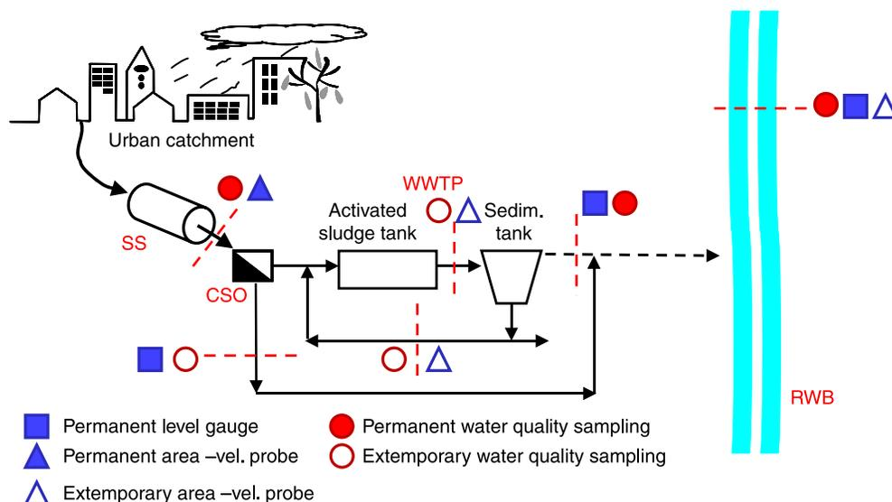
**Figure 3** | Schematic of the urban drainage system monitoring methodology performed on the Montelepre and Giardinello urban areas.
