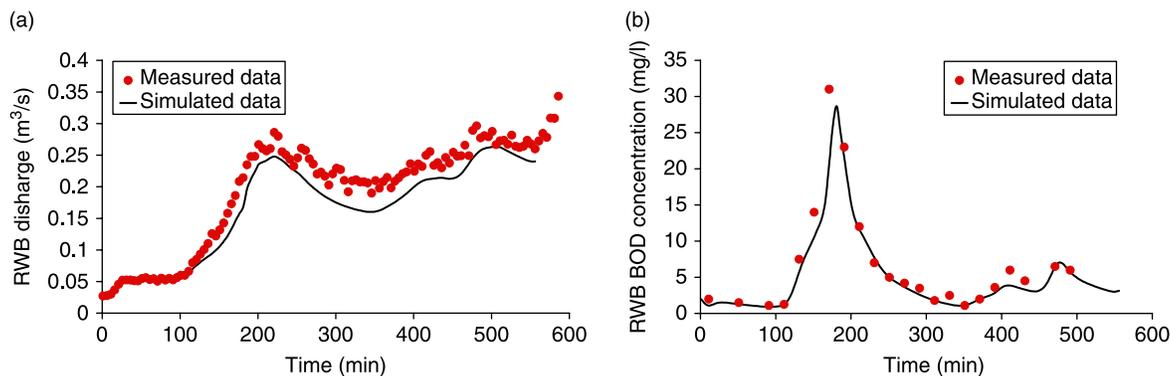
**Figure 7** | Comparison between monitored data and modelling outputs at the "Nocella a Zucco" hydro-meteorological station (event 5/03/2008): river discharge (a) and BOD concentrations (b).
