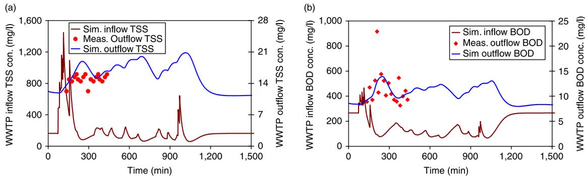
**Figure 6** | Comparison between monitored data and modelling outputs at the Montelepre WWTP (event 5/03/2008): inflow and outflow TSS (a) and BOD (b) concentrations.
