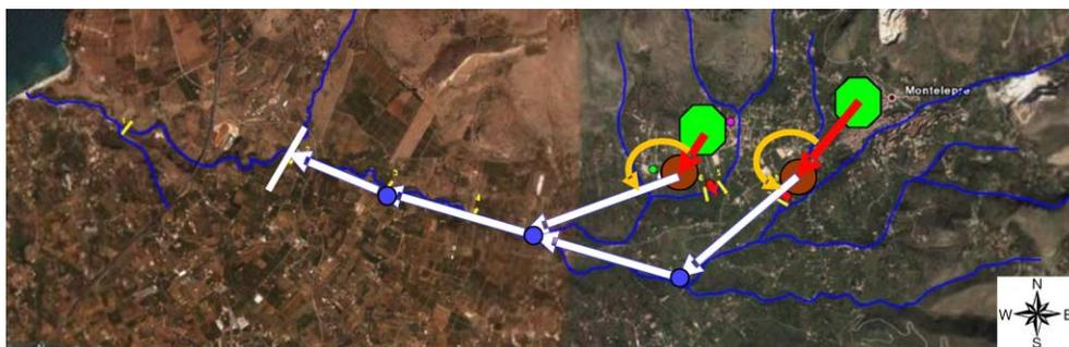
**Figure 4** | Integrated model conceptual scheme indicating two simulated urban catchments (hexagon), two SS (arrow from hexagons), two WWTP (biggest circle), two CSO (semi-circular arrow), and five RWB reaches (linear arrow).
