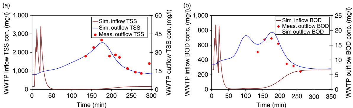
**Figure 9** | Comparison between monitored data and modelling outputs at the Giardinello WWTP (event 27/04/2008): inflow and outflow TSS (a) and BOD (b) concentrations.
