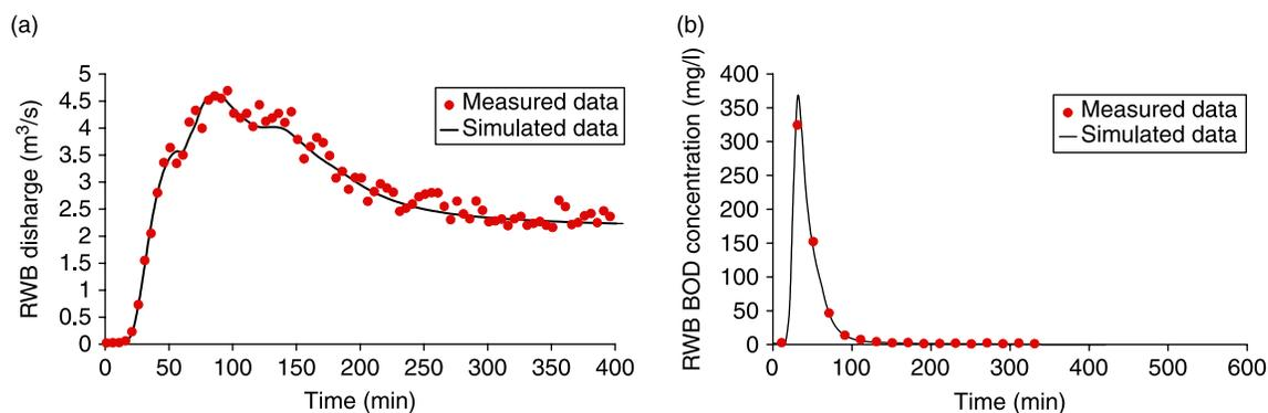
**Figure 10** | Comparison between monitored data and modelling outputs at the “Nocella a Zucco” hydro-meteorological station (event 27/04/2008): river discharge (a) and BOD concentrations (b).
