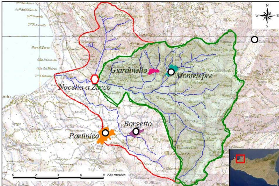
**Figure 2** | Overview of the Nocella basin with indication of the four included urban areas: the monitored sub-catchment is shaded, rain gauges are indicated by white dots, and the flow gauge station is indicated by a white hexagon.
