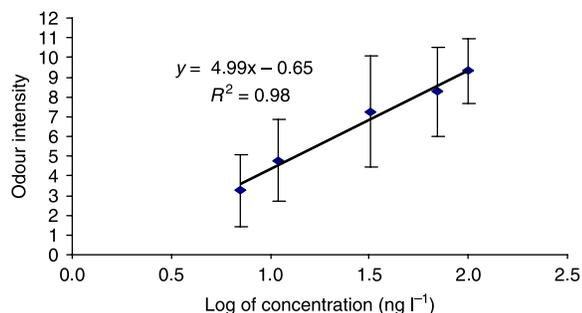
**Figure 1** | Weber-Fechner curves developed in this study for MIB at 45°C.
