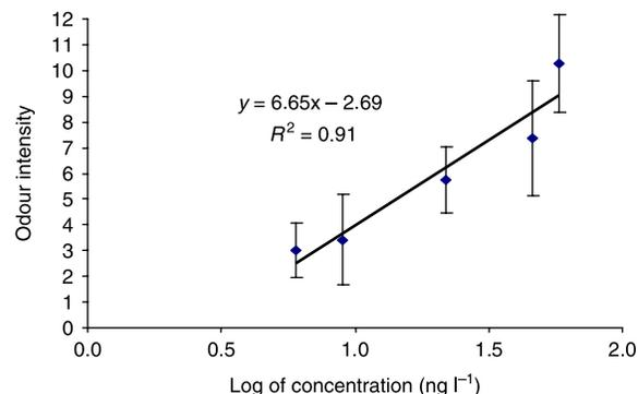
**Figure 2** | Weber-Fechner curves developed in this study for geosmin at 45°C.
