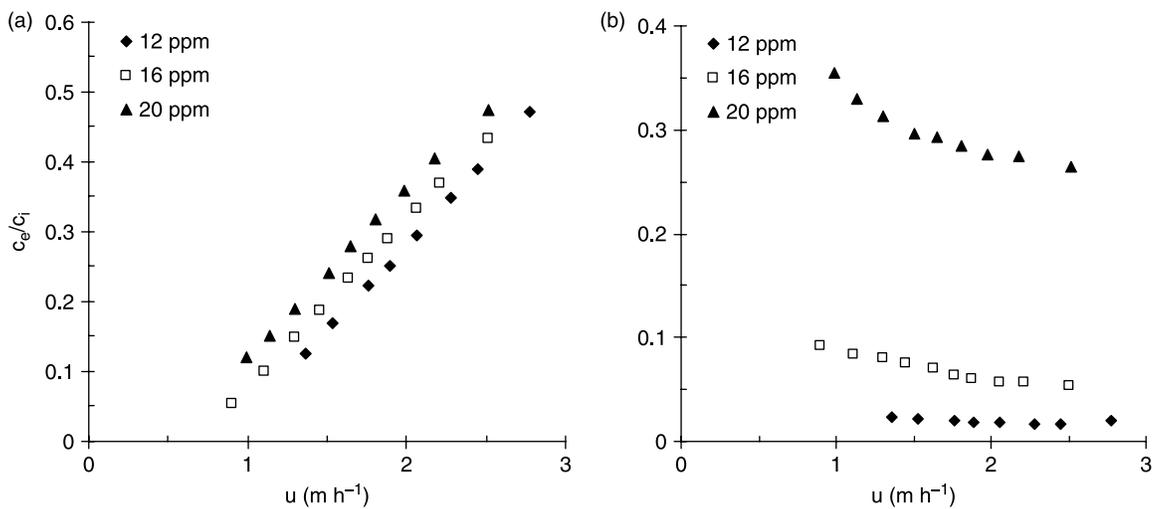
**Figure 5** | (a) capture ratio at  $\alpha = 0.004$  revealing sensitivity to  $G\Phi_F(1 - \Phi_F)L/u$  and (b) illustrating potential impact of floc sizes when  $\alpha$  is defined by Equation (48) with  $d_p = 40 \mu\text{m}$ .
