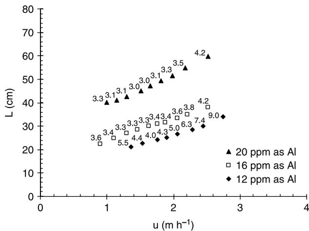
**Figure 2** | Equilibrium heights and effluent turbidities of coagulated suspensions in response to the upflow velocity (Su *et al.* 2004).
