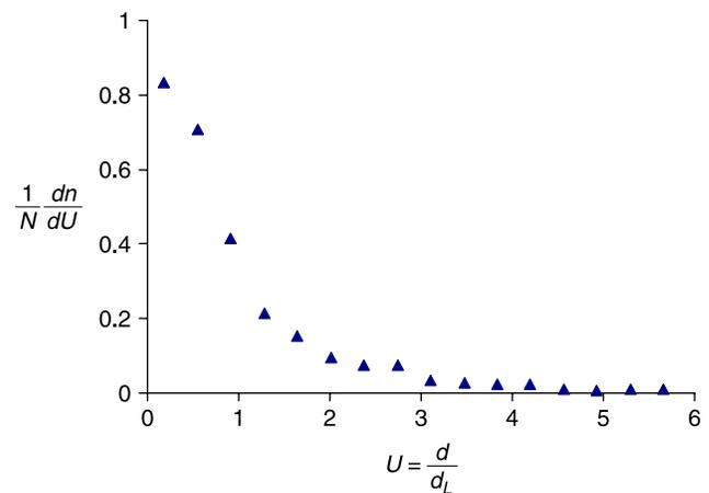
**Figure 1** | Example of floc size distribution from a clarifier receiving a low turbidity coloured water coagulated with alum.  $N$  refers to the total number of flocs per unit volume, and  $dn$  is the number concentration in the interval  $U$  to  $U + \delta U$ .
