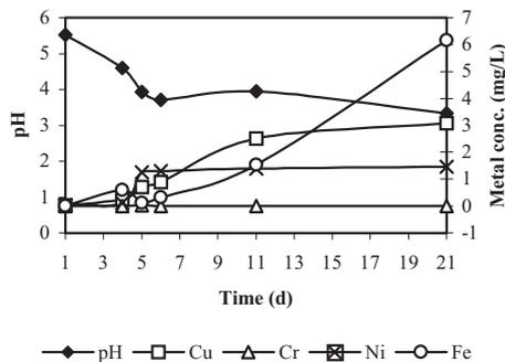
**Figure 3** pH and heavy metal concentrations in sludge in set C
