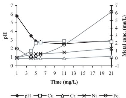
**Figure 1** pH and heavy metal concentrations in supernatant of sludge in set A
