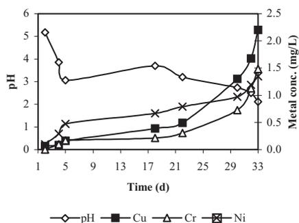
**Figure 2** pH and heavy metal concentrations in supernatant of sludge in set B
