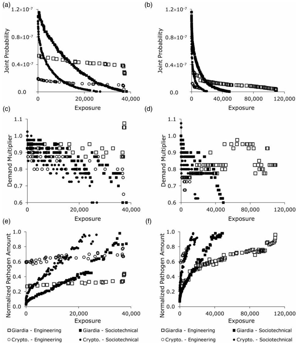
**Figure 7** | Multi-objective optimization results for contamination of West WTP (left column) and East WTP (right column); (a) and (b) illustrate maximum-risk frontiers, (c) and (d) show demand multiplier associated with scenarios in maximum-risk frontiers, and (e) and (f) indicate injected pathogen amount associated with scenarios in maximum-risk frontiers.
