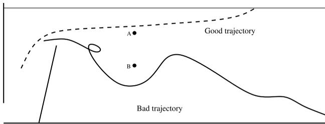
**Figure 1** | Schematic of a second generation dissolved air flotation tank. The dashed line represents the path of a bubble/particle agglomerate that leads to successful flotation, the solid line corresponds to unsuccessful flotation.
