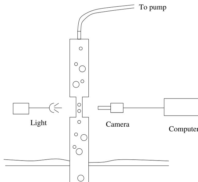
Figure 3 | Schematic of bubble size distribution instrumentation.
