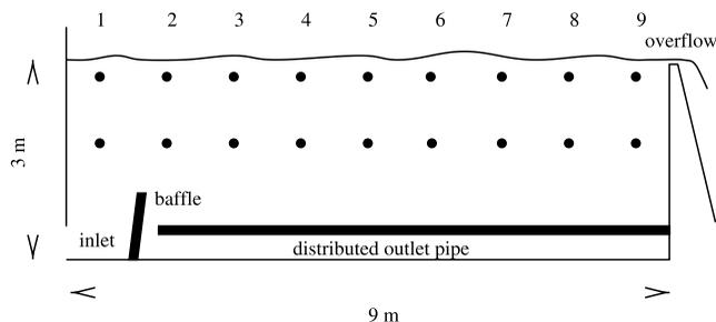
Figure 5 | Location of the measurement points during the Graincliffe study.
