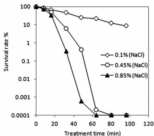
**Figure 3** | Effects of NaCl concentration on the bactericidal properties of the BDD disinfectant against *E. coli*. The water flow rate was fixed at 250 mL min<sup>-1</sup> and a voltage of 3 V was used in the electrolytic process.
