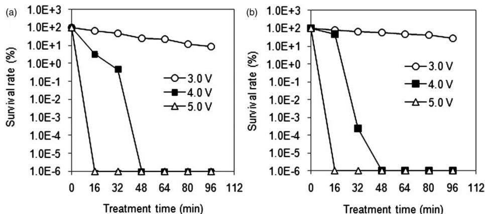
**Figure 2** | Effects of voltage on the bactericidal properties of the BDD disinfectant against (a) *E. coli* and (b) *P. aeruginosa*. The flow rate was fixed at  $250 \text{ mL min}^{-1}$  and 0.1% NaCl solution was used as the electrolyte in each test.
