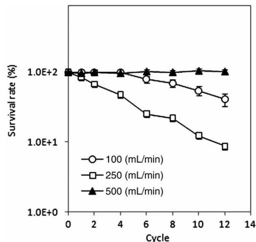
**Figure 4** | Effects of flow rate on the bactericidal properties of the BDD reactor against *E. coli*. The concentration of NaCl solution was controlled at 0.1% and a voltage of 3 V was used in the electrolytic process.
