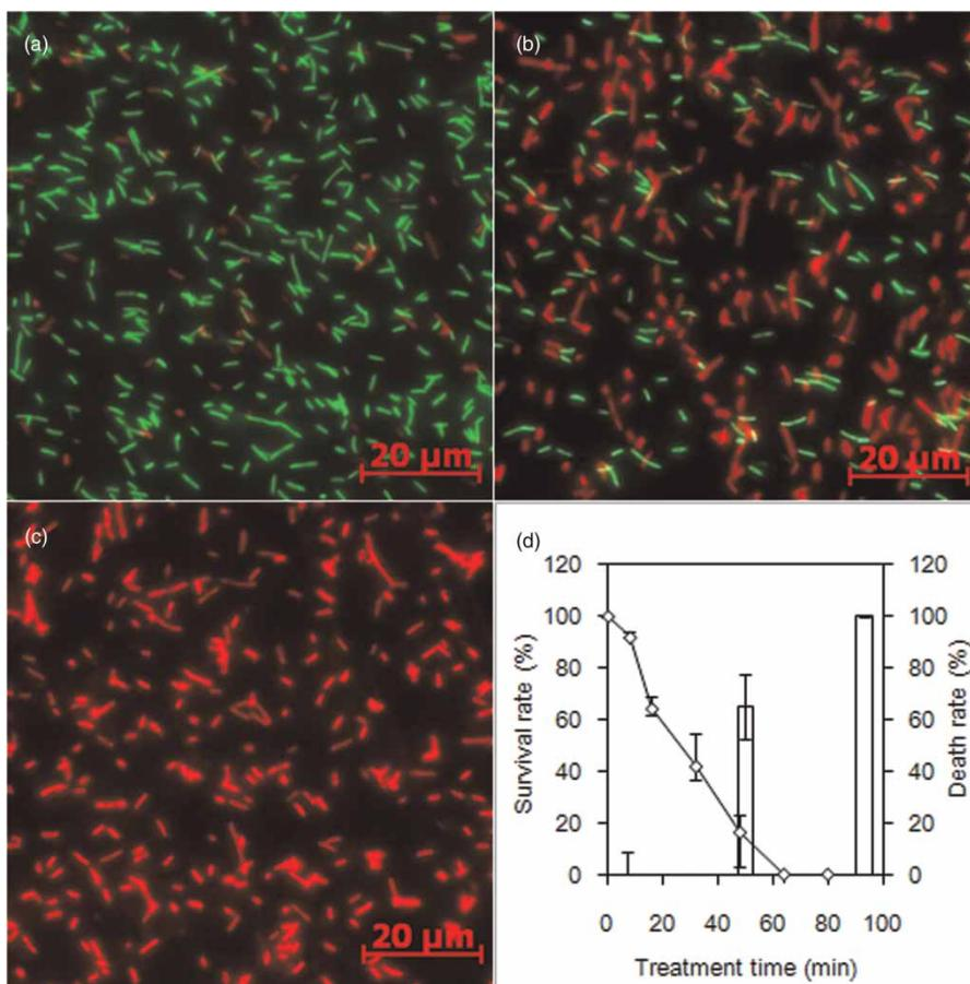
**Figure 6** | Bactericidal effect of the BDD reactor on *L. pneumophila* in water samples treated with a 4.0 V voltage and a  $250 \text{ mL min}^{-1}$  flow rate. (a), (b) and (c) indicate the representative fluorescence microscopy from 0, 32 and 80 min of treatment, respectively. (d) Shows the survival and death rates of *L. pneumophila* obtained by ( $\diamond$ ) the colony formation method and ( $\square$ ) quantitative fluorescence microscopy analysis.
