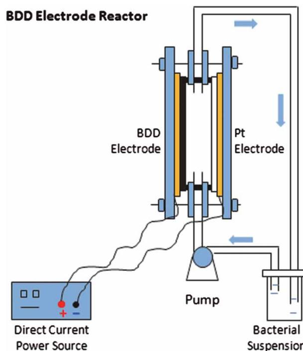
Figure 1 | Illustration of the BDD electrode reactor.
